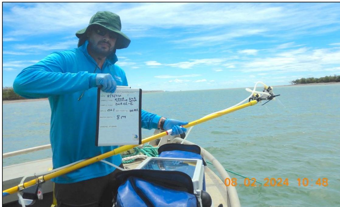
Figure 2. Water sampling with telescopic pole.
