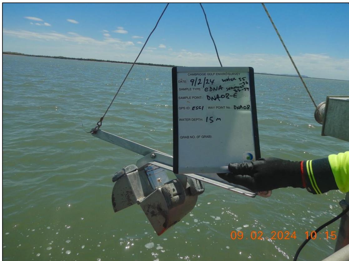
Figure 3. Grab used for taking seabed sediment samples.
