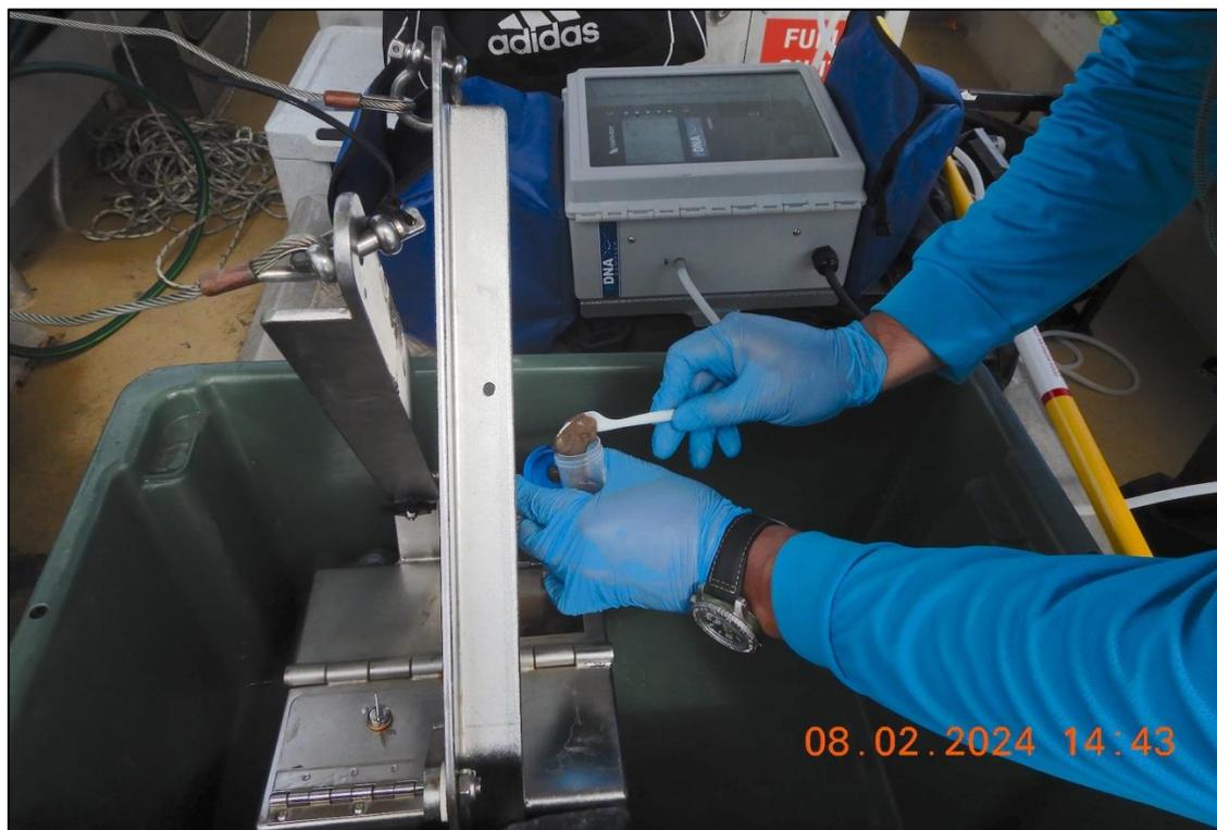
**Figure 4.** Taking sediment samples from the grab.
