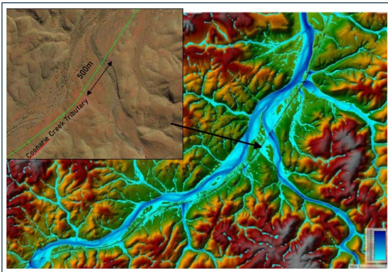
Figure 4 Crossing 2 - Alignment 1B in parallel to main Coonarie Creek Tributary (flood map from Calibre 2022b)
