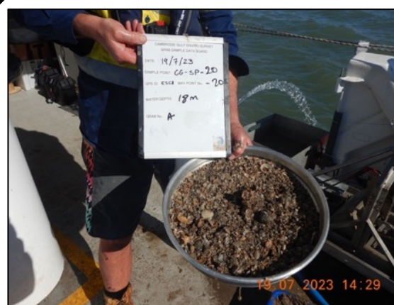
FIGURE 6.25: Two examples of the photographic record of the grab sampling procedure used for both the dry- and wet-season sampling. Note the sample on the left is the typical sand that is found throughout CG, which typically left very little material after sieving, as per the lower left image. The sample on the right is clay/shell grit, which typically left a larger volume of material after sieving, as per the lower right image.
