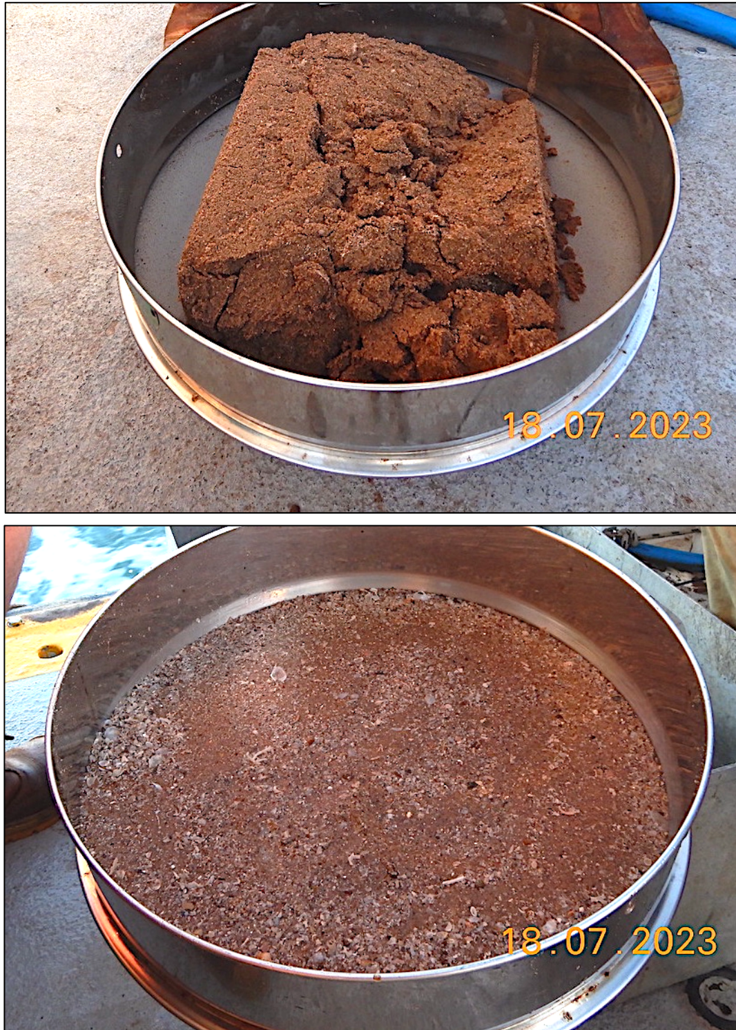
FIGURE 6.40: An example of a grab sample of sand from within the proposed operational area. Top is pre-sieve and bottom is post-sieving to 500 microns, which was then searched for biota. Most sand samples did not contain biota, as constant movement of the sand under tidal currents prevents colonization. Compare this with Figure 6.42.
