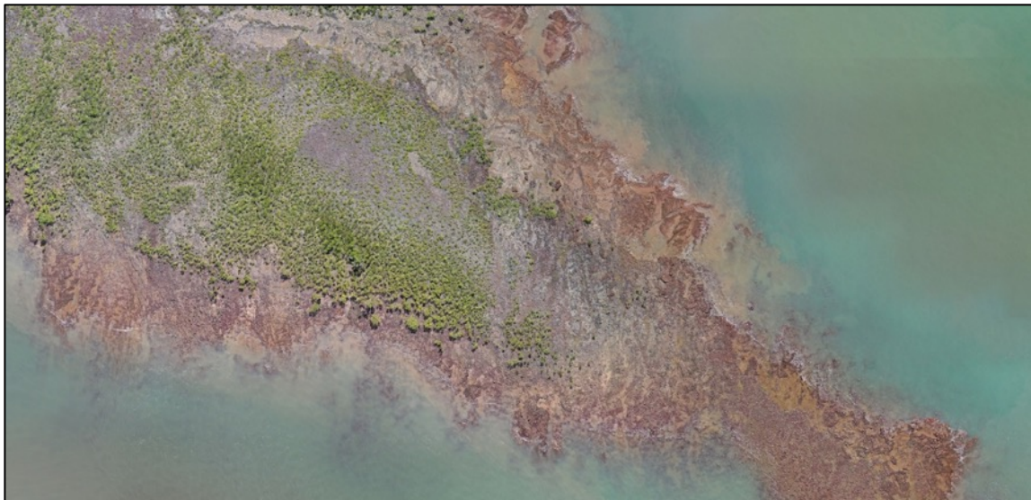
FIGURE 6.15: An example of an orthomosaic of an intertidal rocky substrate site, created from the fine-scale vertical imagery. The original images are extremely high-resolution allowing zooming-in to assess details in the cm range. This site is Vancouver Point / Myrmidon Ledge as marked on Figure 6.7 – Left.
