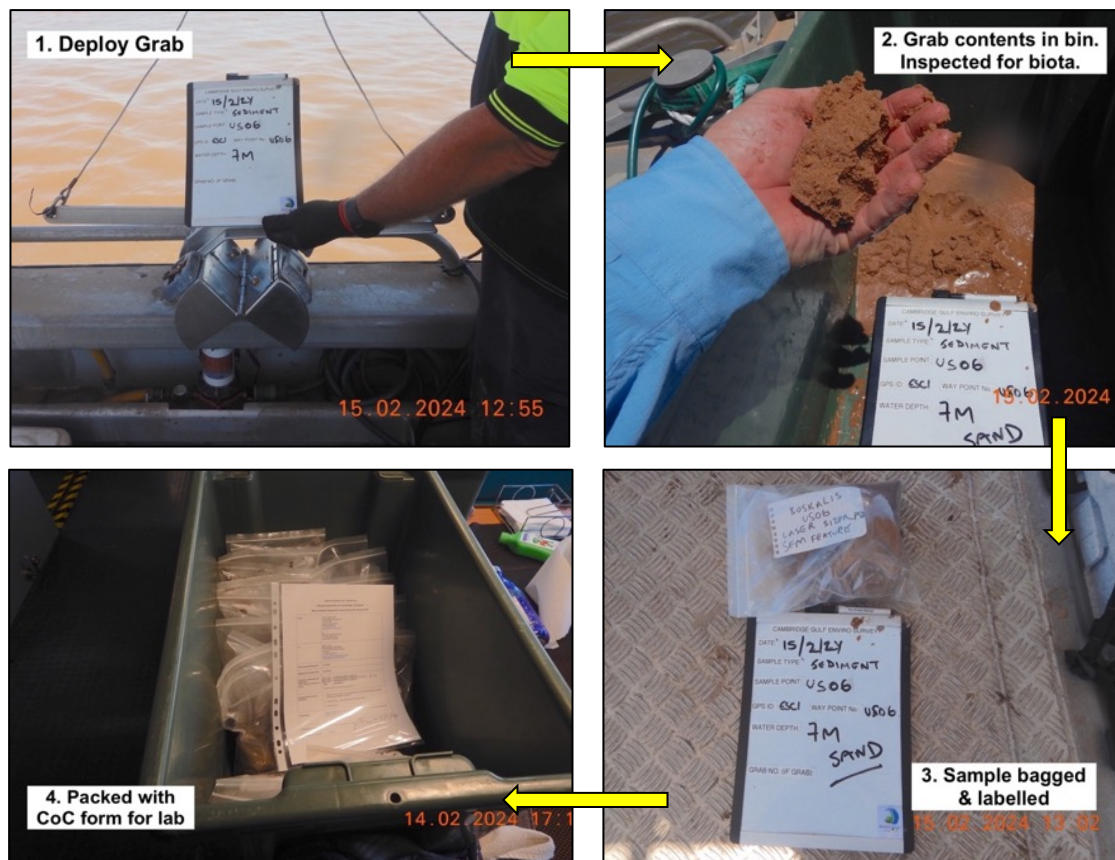
FIGURE 6.32: Sediment grabs. For quality control and sample chain of custody, each step of the process was photographed. This site (US06 – see Figure 6.33) is in the headwaters of CG (Pentecost River). All samples in that area were sand / sand-mix, with the same characteristics as the sand in CG, as per top right image. This indicates the upstream source of the sand in CG.
