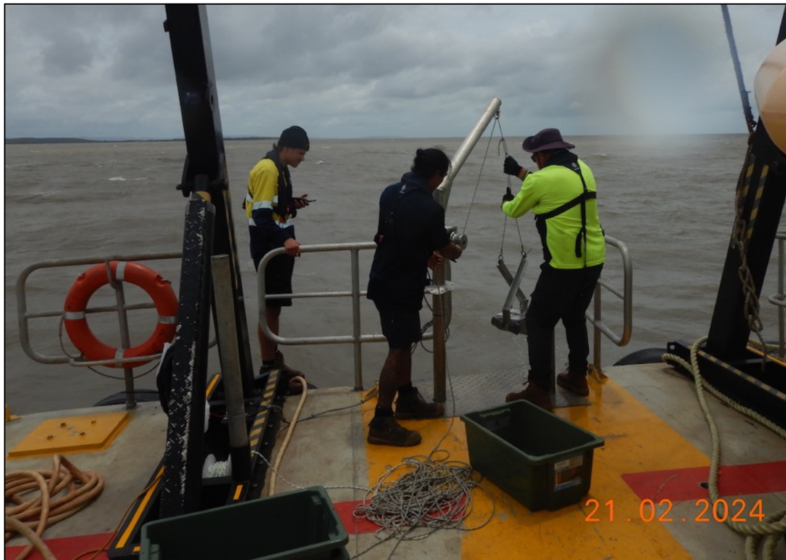
FIGURE 6.23: Grabs were deployed and recovered by electric or hydraulic winch depending on the vessel.
