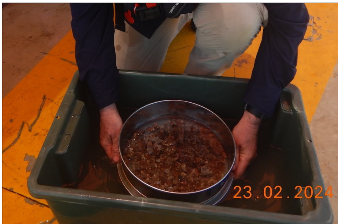
FIGURE 6.30: For courser sediments like shell-grit and gravel, after initial sieving and biota assessment, the sieve and retained sediment was returned to a bin of seawater with the water ~0.5 to 1 cm above the sediment surface, then gently shaken. This 'floated off' any small organisms that might have been missed visually amongst the sieved sediment.
