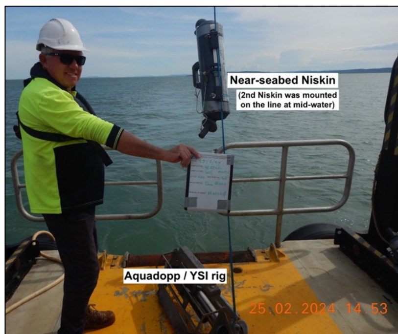
FIGURE 8.9: Equipment set-up for Vertical Water Quality Profile sites in CG wet season Feb 2024, with near-seabed Niskin shown. A second Niskin was fitted to the line at the mid-water point as the rig was lowered to the seabed.
