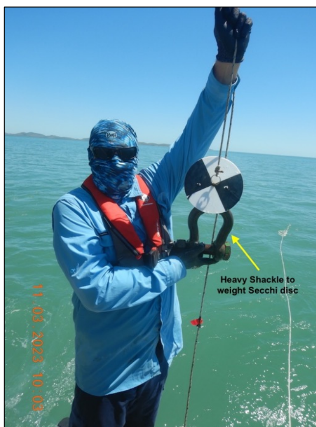
FIGURE 8.2: The Secchi disc used. Note the heavy shackle to drop the disc vertically in strong tidal currents.
