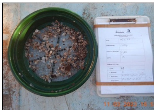
FIGURE 6.21: Two examples of the photographic record of each step in the grab sampling procedure. The full set of photographs for all 18 sites sampled in March 2023 is archived, and can be provided to regulatory agencies if required.
