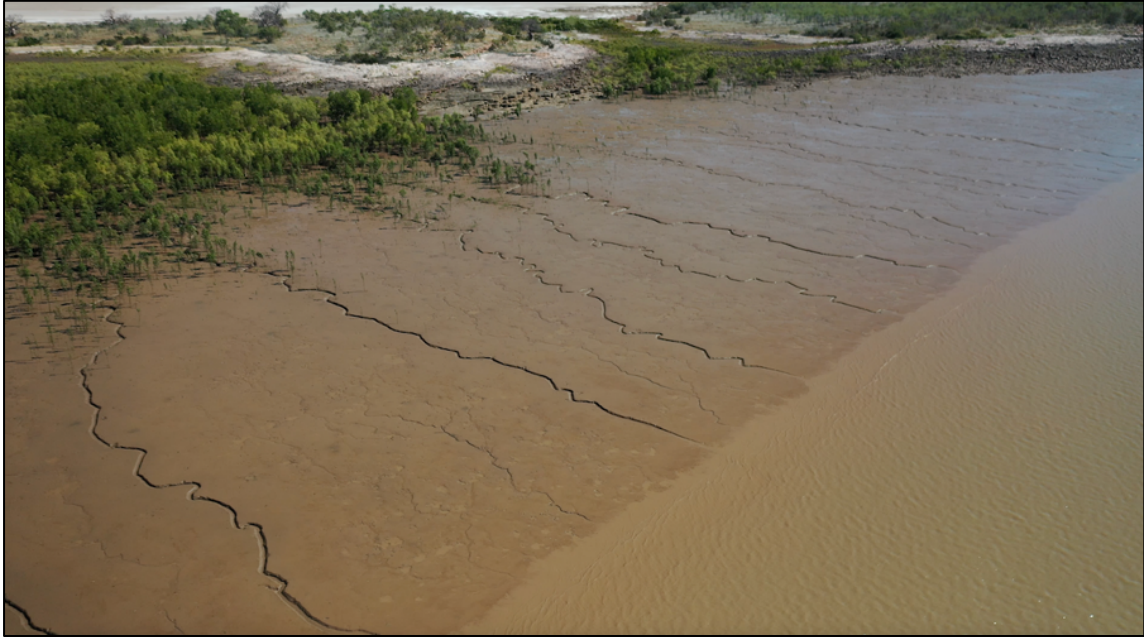
FIGURE 6.12: An example of oblique aerial drone imagery of intertidal mudflats. Any indications of seagrass or other benthos such as colouration, were investigated in detail by the drone. Fine-scale vertical images were also taken. This site is 'Nicholls Point SW' as marked on Figure 6.7 – Right.
