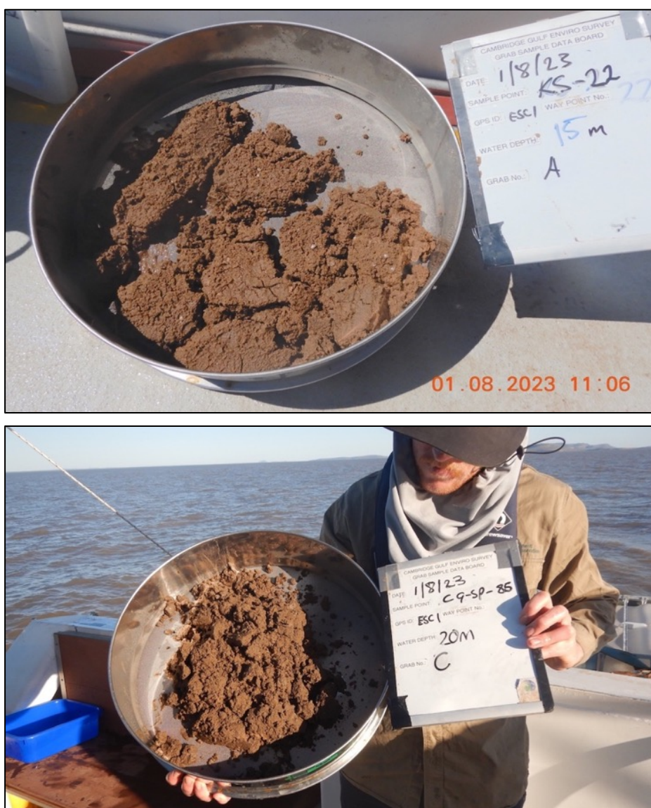
FIGURE 5.9: Examples of the sand found in Block 4 using a Smith-McIntyre Grab during the environmental survey in Jul-Aug 2023. Note the coppery-brown colour is similar to the source rocks in the catchment shown in Figure 5.2 (images: Raaymakers).
