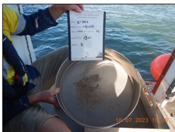
FIGURE 6.25: Two examples of the photographic record of the grab sampling procedure used for both the dry- and wet-season sampling. Note the sample on the left is the typical sand that is found throughout CG, which typically left very little material after sieving, as per the lower left image. The sample on the right is clay/shell grit, which typically left a larger volume of material after sieving, as per the lower right image.
