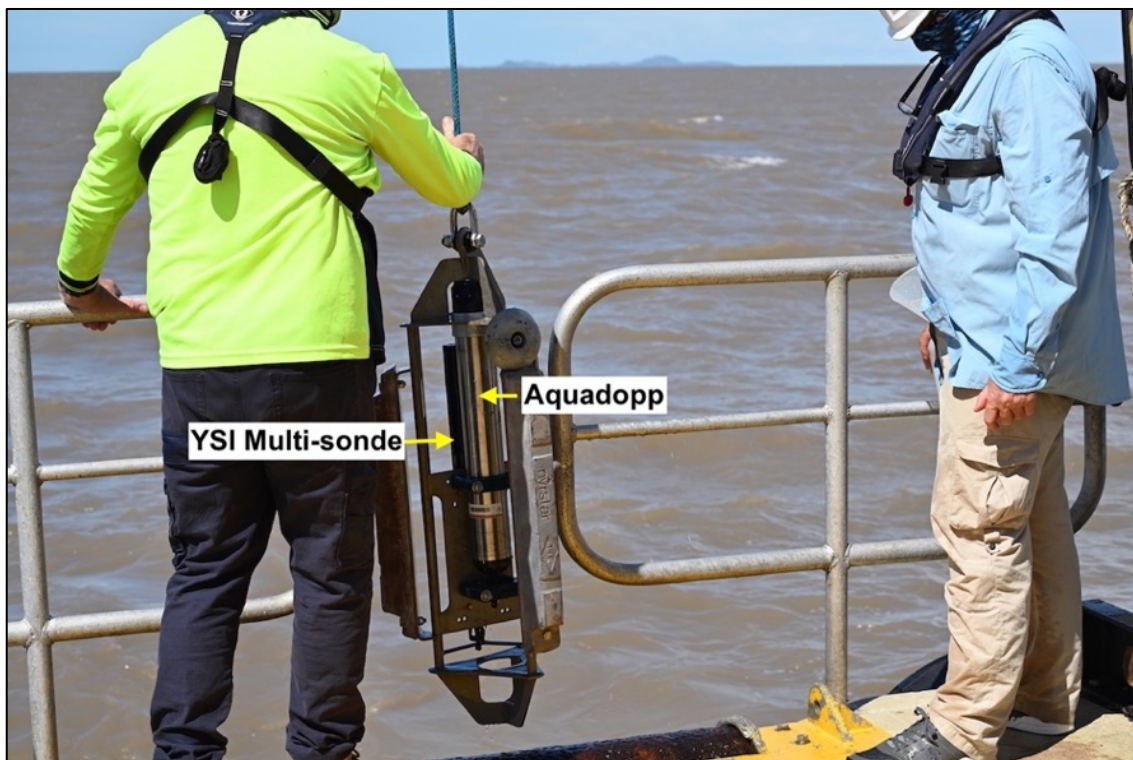
FIGURE 8.8: Equipment set-up for Vertical Water Quality Profile sites in CG wet season Feb 2024 (Niskin not shown)
