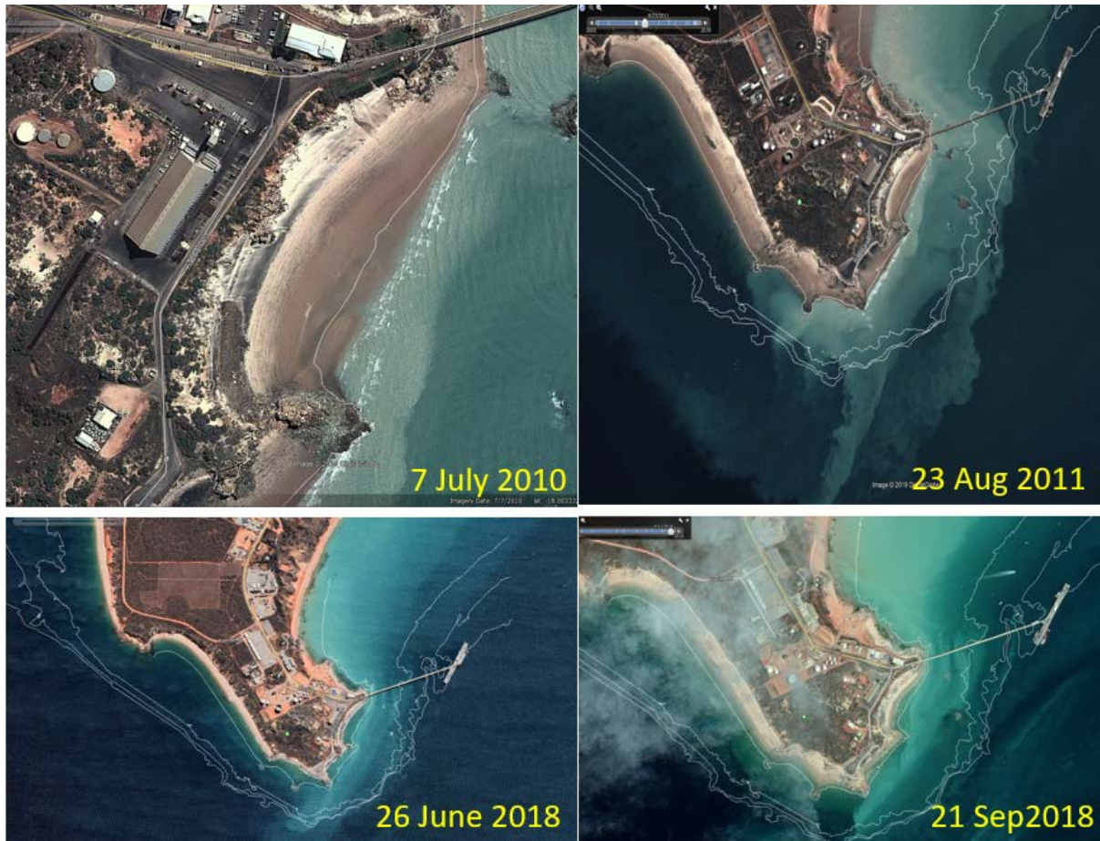
Figure 8.4: Selection of photos from Dry Season Months showing suspended sediment in the water column moving around Entrance Point (Google Earth)
