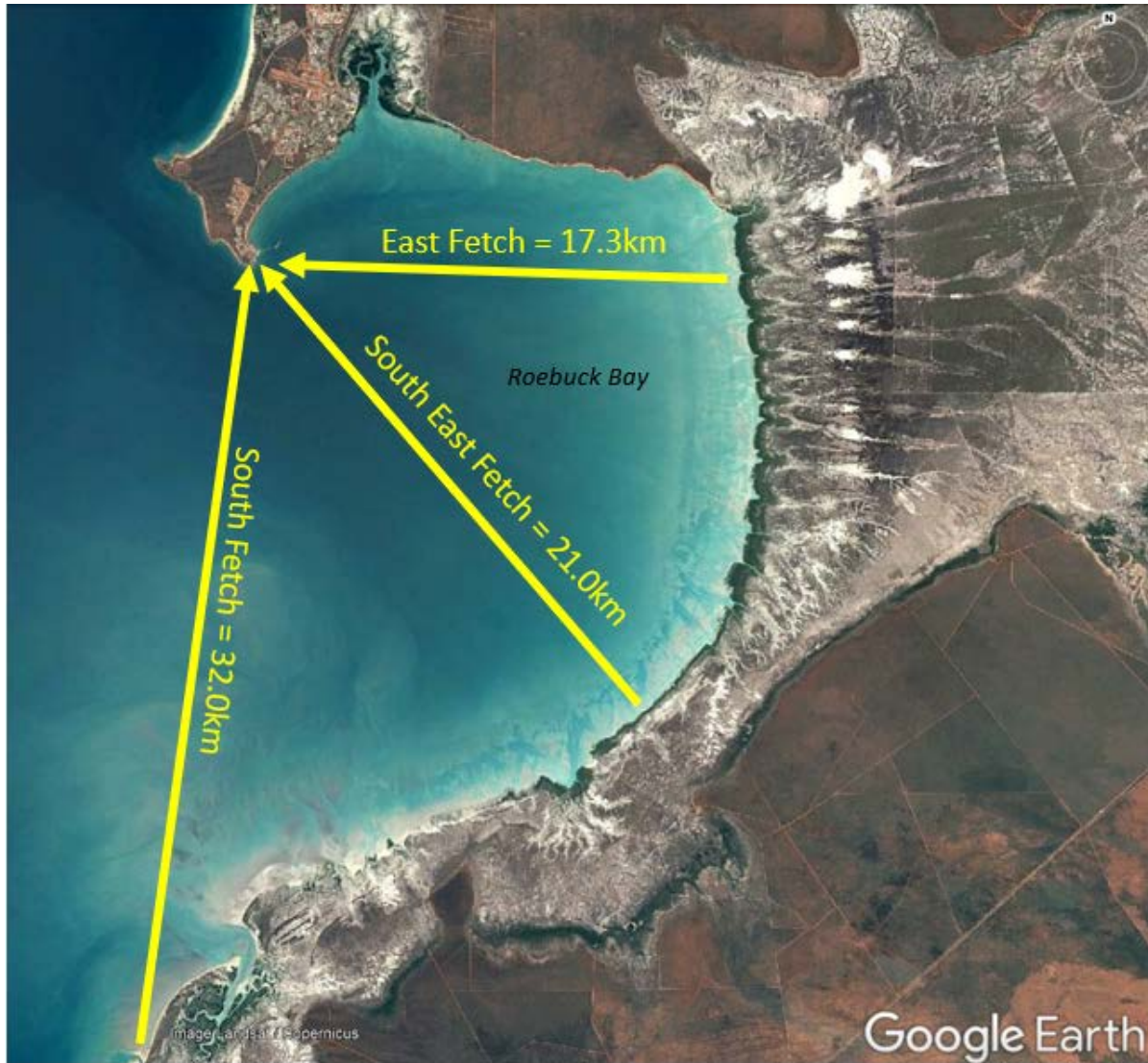
Figure 3.6: Fetch Distance across Roebuck Bay for key wind directions affecting wave propagation to the site (Google Earth)
