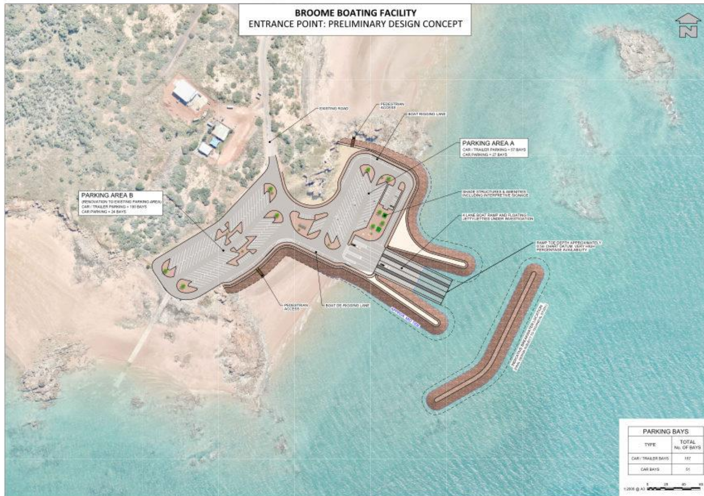
Figure 1. Proposed Broome Boating Facility design concept and infrastructure layout, located at Entrance Point, Broome, south of the Broome Jetty.
