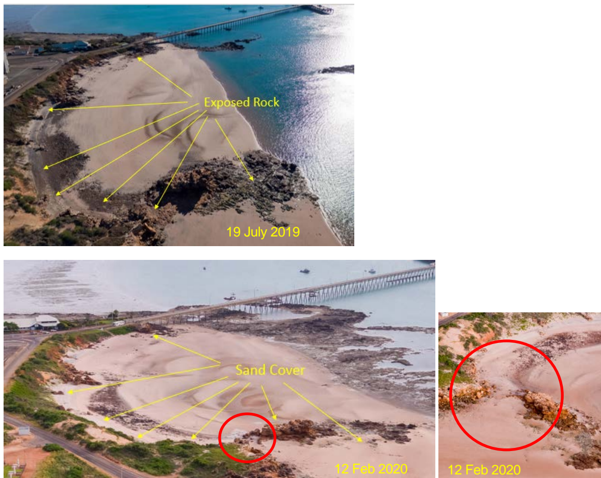
Figure 8.11: Comparison of drone images north beach compartment – Upper Photo 19 July 2019 (mid Dry Season), Lower photo 12 Feb 2020 (mid-Wet Season). In dry season the upper beach is exposed rock (July 2019). The rock is then overlain with sediment by late wet season (Feb 2020).
