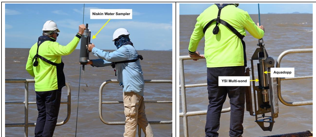
Figure 25. Setup for the water column profiling equipment. Included two Niskins, one near seabed above the Aquadopp and Multi-sonde frame (right image), and one at mid water (the midwater Niskin is shown in left image before deployment).
