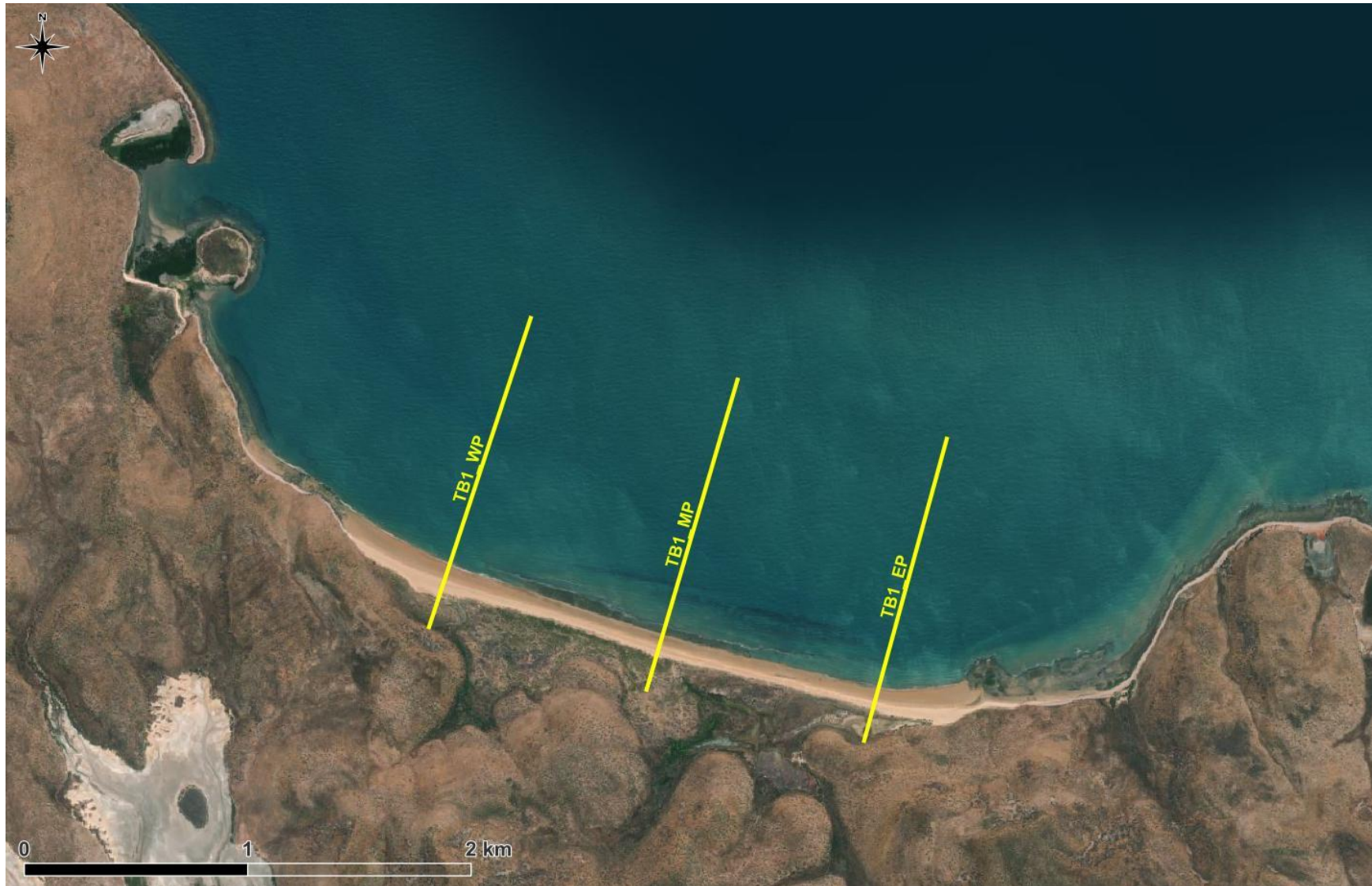
Figure 60. Cross-shore profiles adopted to assess historical shoreline change at Turtle Beach West using CoastSat.
