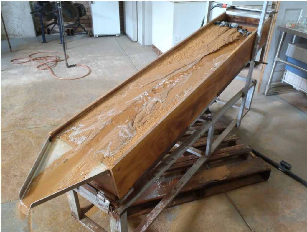
Plate 4.3: Laboratory-scale, rill erosion flume
