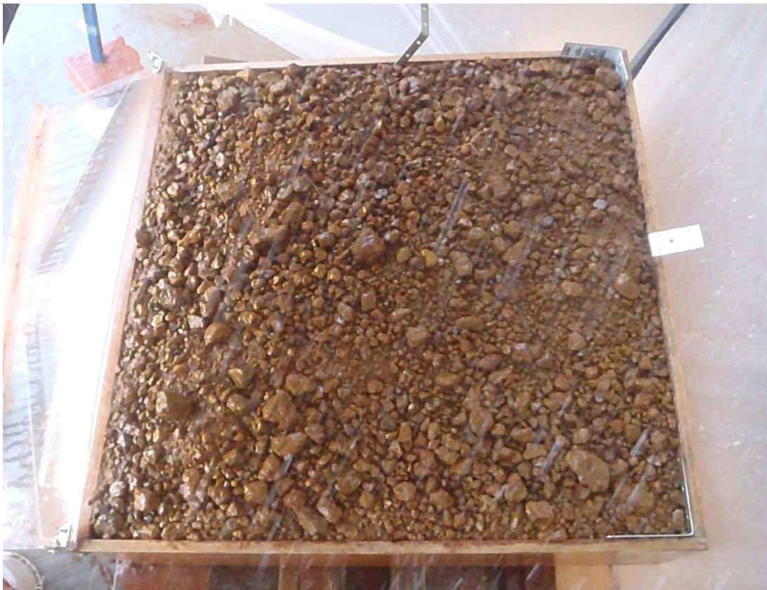
Plate 4.4: Self-armouring of gravelly material during erosion testing
