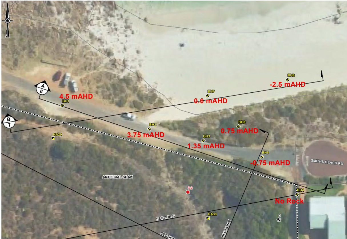
Figure 3.6 Spatial View Showing Elevations of Rock Observed in Boreholes
