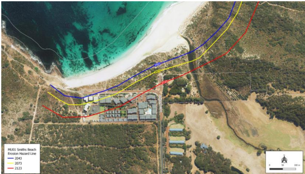
Figure 2.1 Coastal Erosion Hazard Lines (City 2022)
