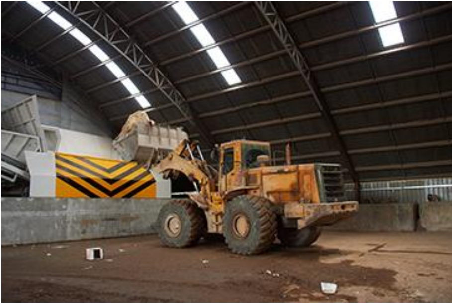
Figure 1: Mixed waste from IWM is dropped onto the apron feeder for sorting at the Bayswater MRF
