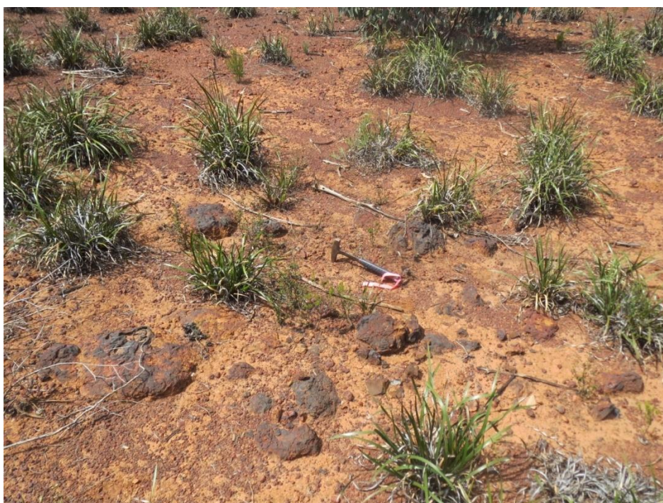
Plate 5: Lateritic Pyroxenite Cover Material
