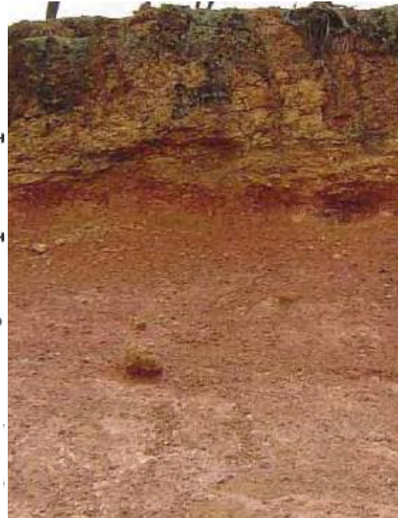
Figure 1. Typical lateritic profile in the south west of Western Australia (from Moore, 2011 (left) and Sawkins, 2011 (right)).
