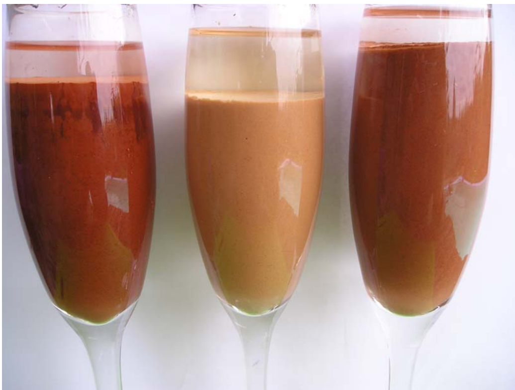
Picture 19: L to R: Mulga silt, Woodie Woodie, mixed mulga and Woodie Woodie. There is no difference visible in the soil fractions from the two areas when mixed and allowed to settle.
