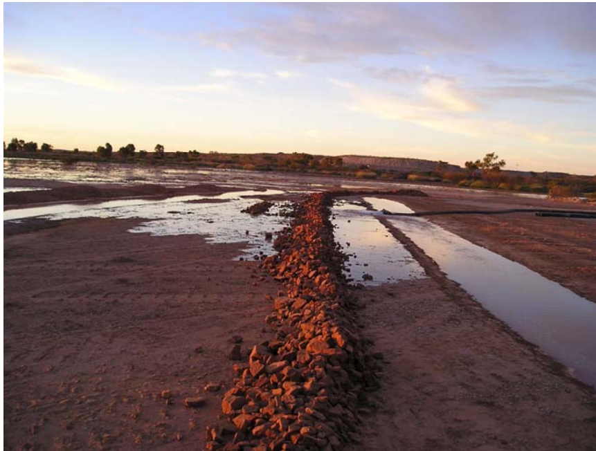
Picture 9: Levee in early stages of discharge at 24.7 l/sec. Note that the ditch has water in it, but that the spread of water along the levee is due to the levee itself.
