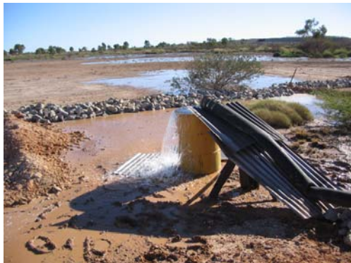
Picture 2: Determining flow rate for various valve settings
