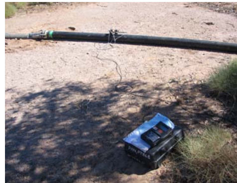
Picture 3: Direct flow measurement with flow meter
