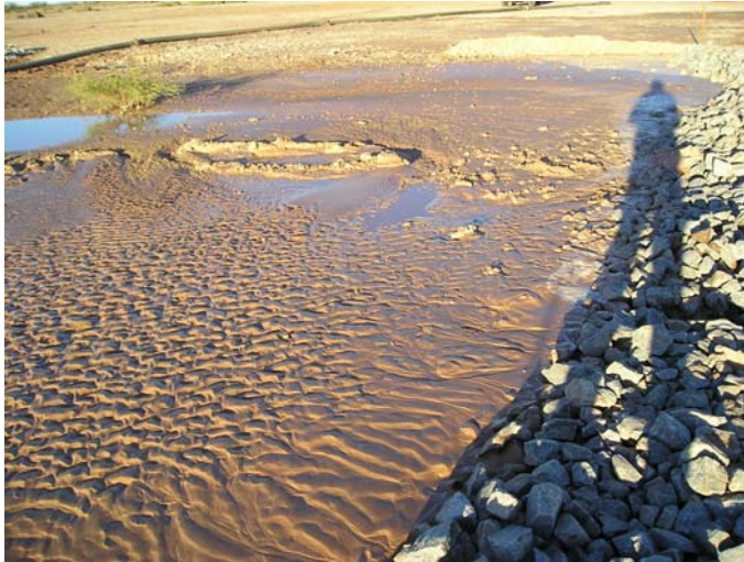
Picture 16a and 16b: Silt in levee after sedimentation trial
