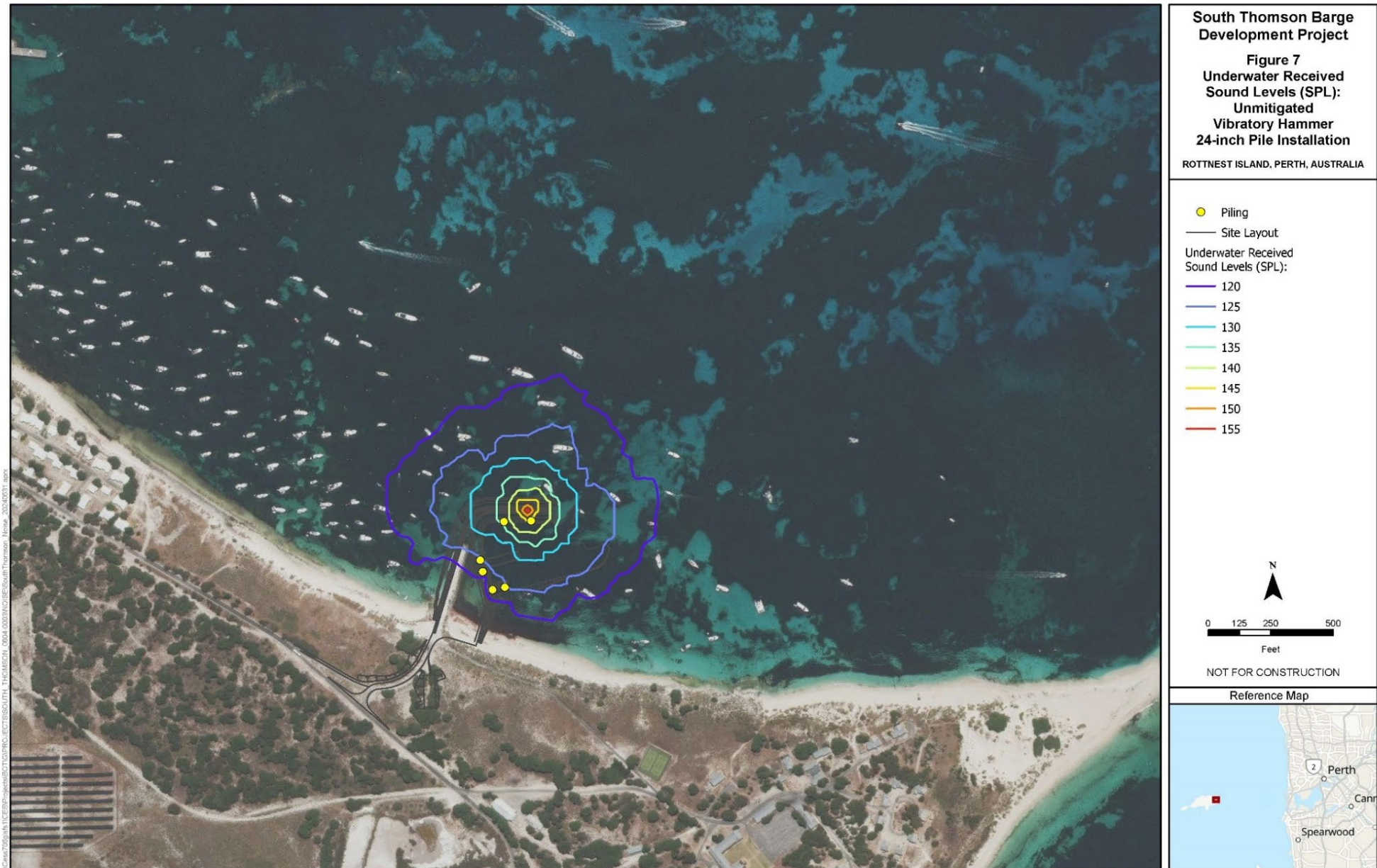
Figure 40: Underwater Received Sound Levels (SPL): Unmitigated vibratory 24-inch pile installation (proposed piling method)
