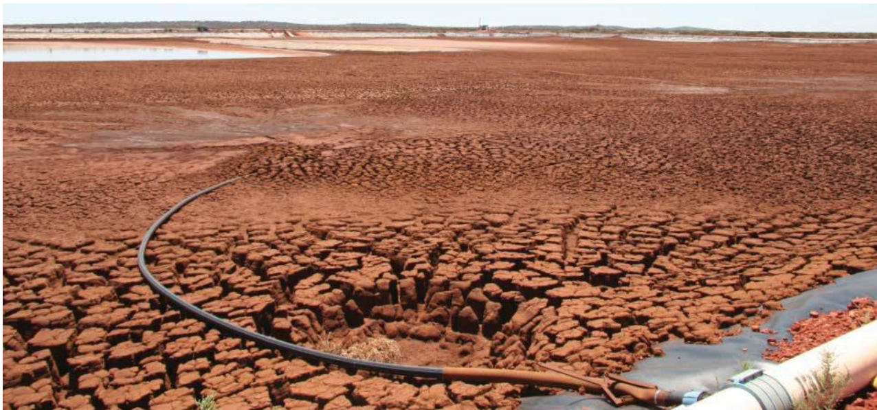
Plate 9-1: Exposed Beach and Spigot in TSF 1 (Hatch 2017)
