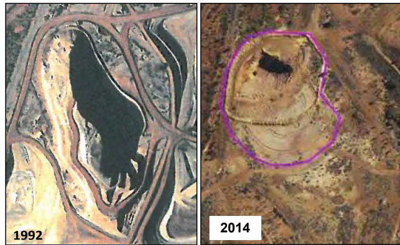
Figure A40: Sir John Open Pit Feature (showing extent of backfill)
