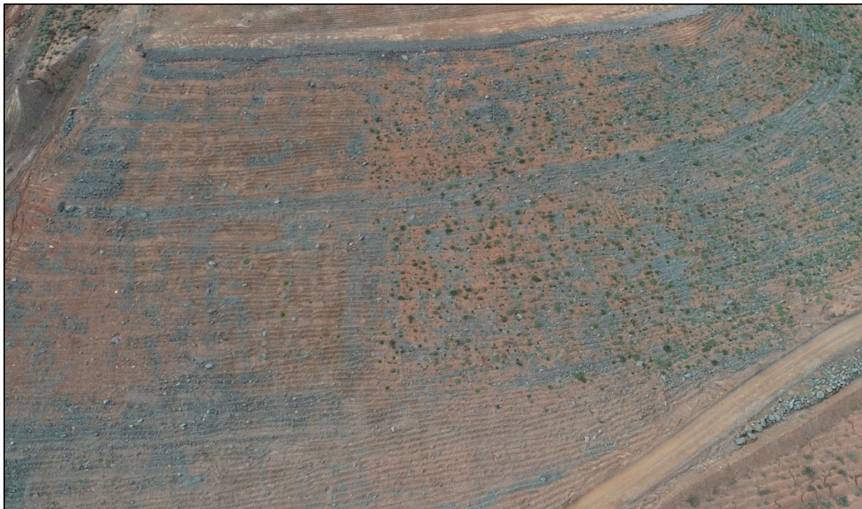
Figure 5-34: Radio Hill (2019) after remedial works (note vegetation difference between Class D (left) and Class A (right) soils)
