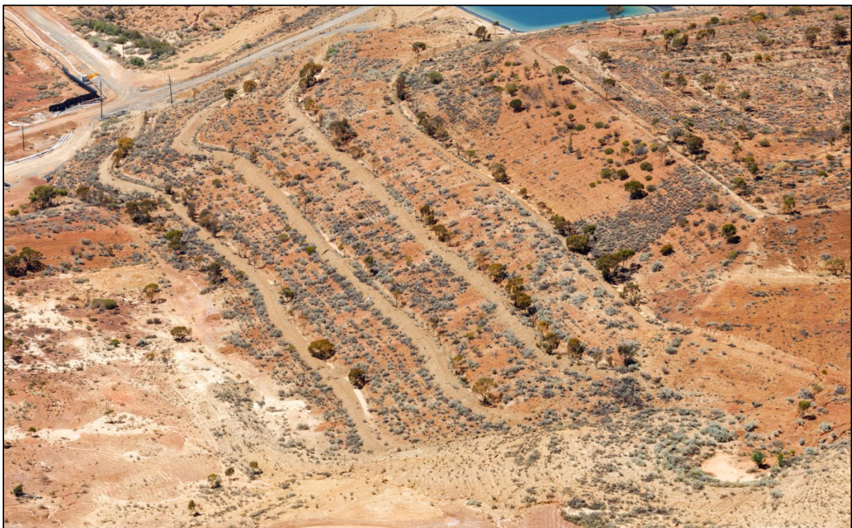
Figure 5-99: Sir John WRD Western Batter Progress of Rehabilitation
