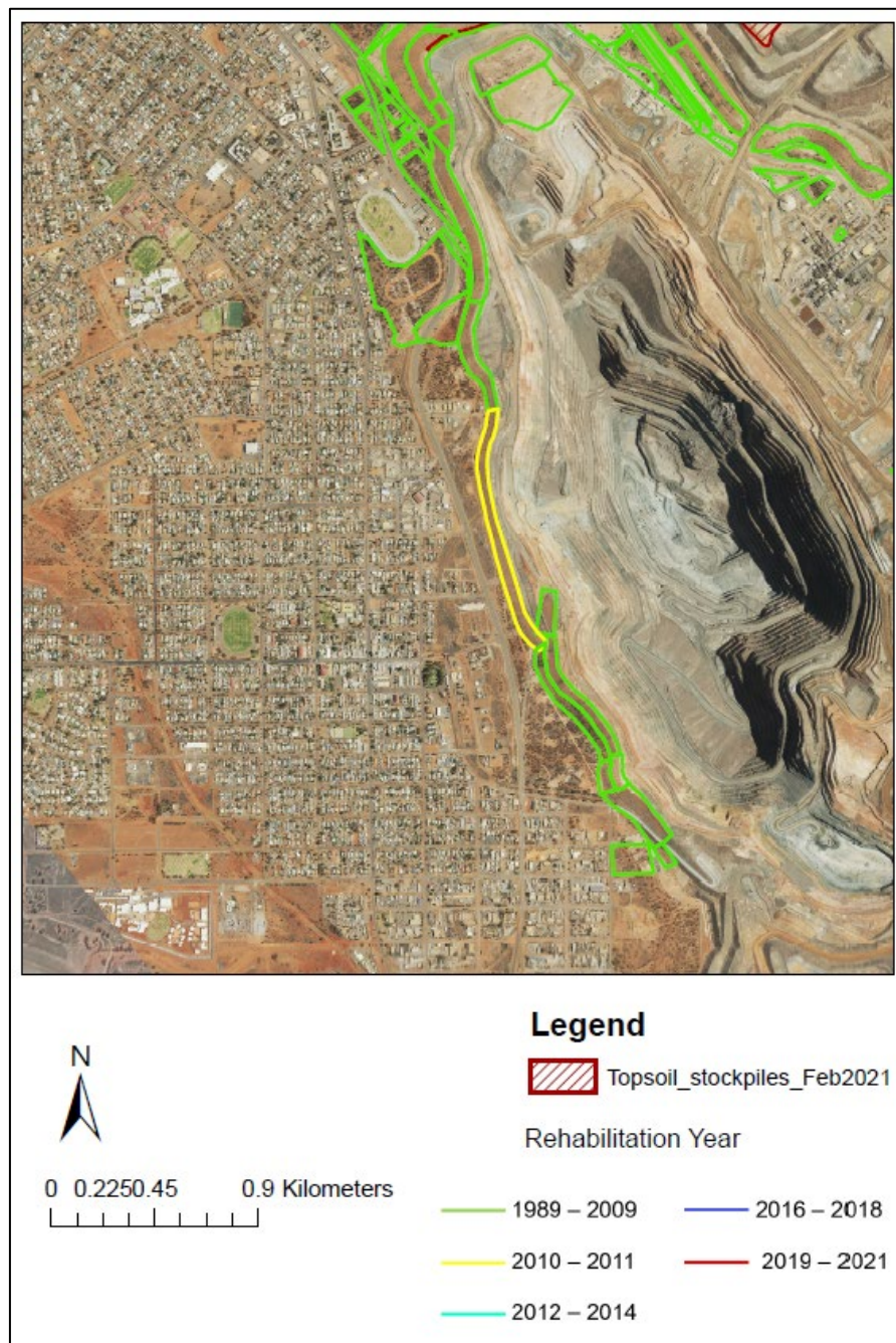
Figure 5-50: Environmental Noise Bund Current Rehabilitation Status (2021)
