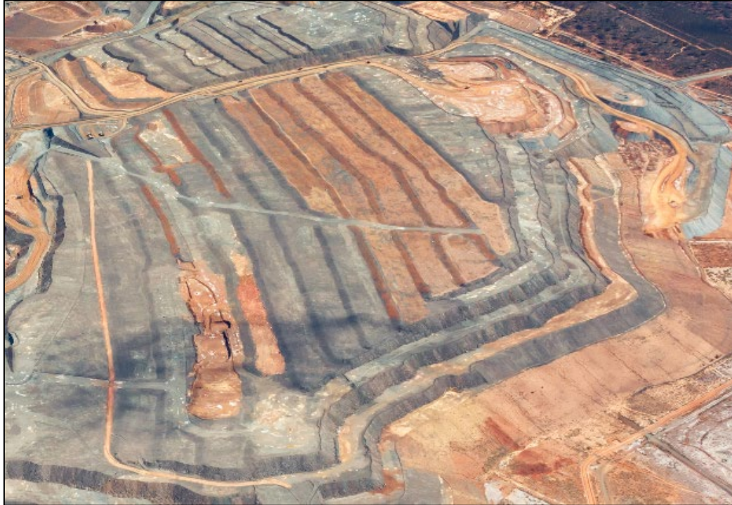
Figure 5-27: 5 m Lift Rehabilitation (2021)
