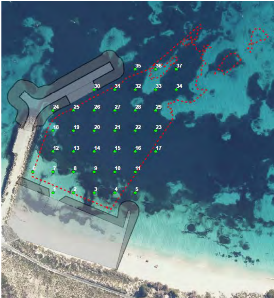
Figure 1. Army Jetty, South Thompson Bay. Marine Magnetic survey to cover the proposed dredge areas (red boundary).
