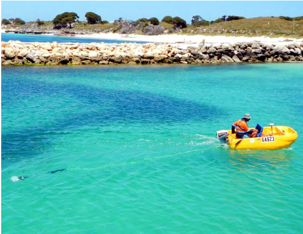
Figure 4. Survey tender with low magnetic properties towing the magnetometer.
