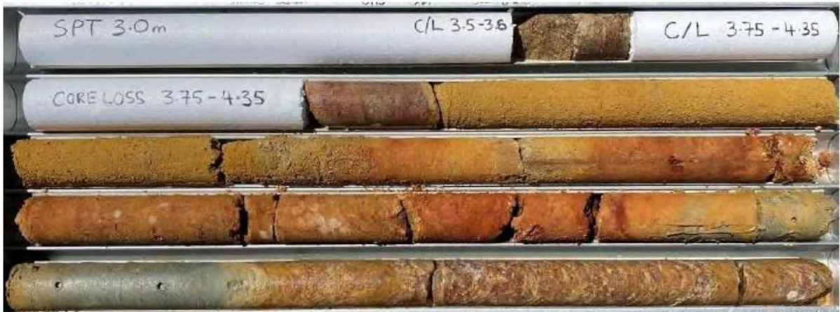
Figure 7. Core photograph BH5, 0-8m.
