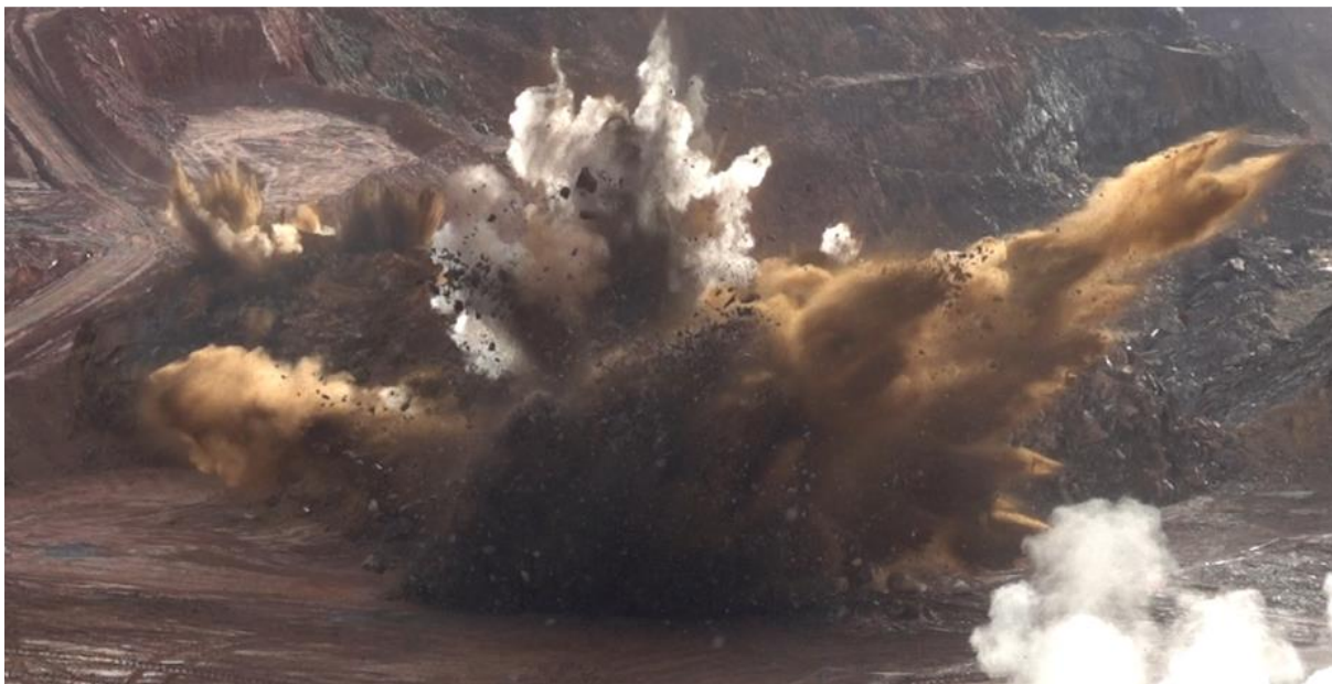
Approx. 100% Cratering Incidence, Intensity Rating 5: 100-1705B.mp4
