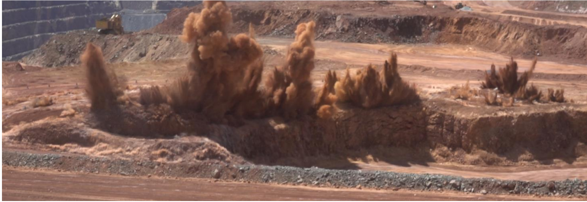
Approx. 10% Cratering Incidence, Intensity Rating 3: 90-1703B04_B07A.mp4
