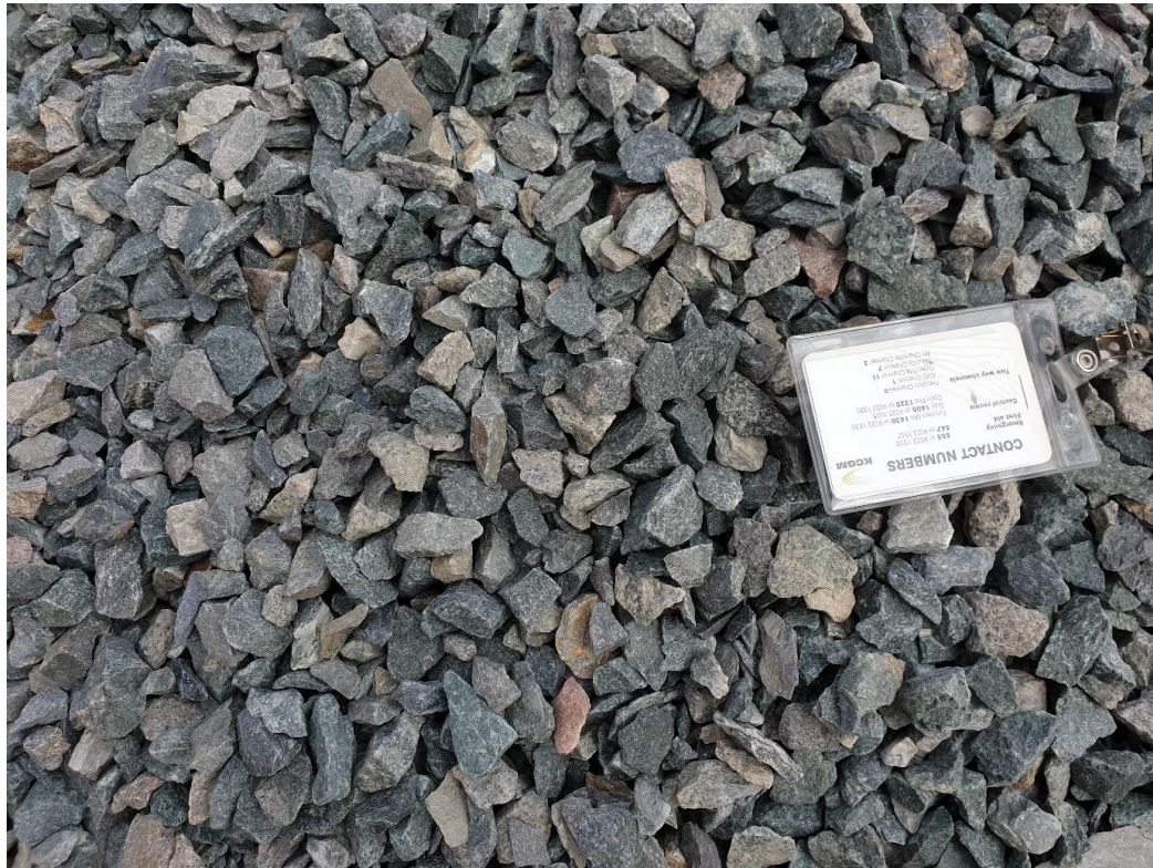
Figure 3. Stemming materials used in all KCGM blasts.
