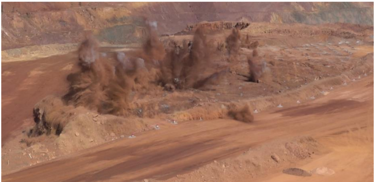
Less than 5% Cratering Incidence, Intensity Rating 3: 80-1707B-09B.mp4
