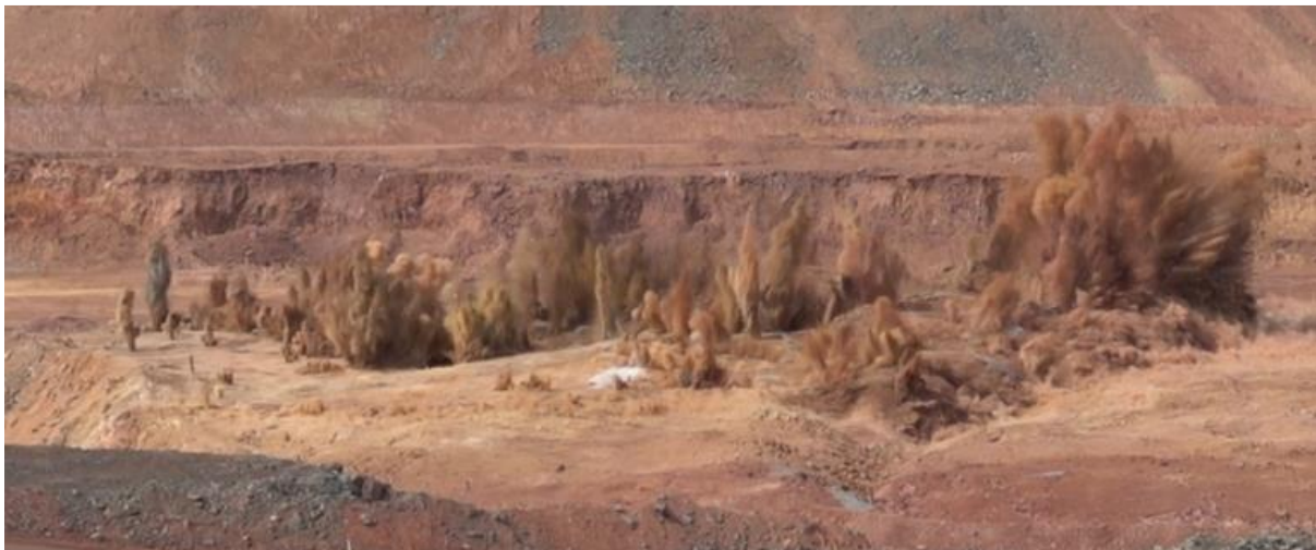
Approx. 20% Cratering Incidence, Intensity Rating 2: 90-1707c.mp4
