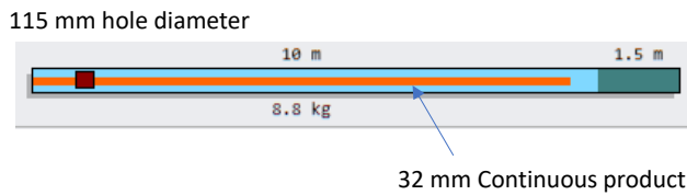
Figure 9. Pre-split charge configurations for benches above the -170 level.
