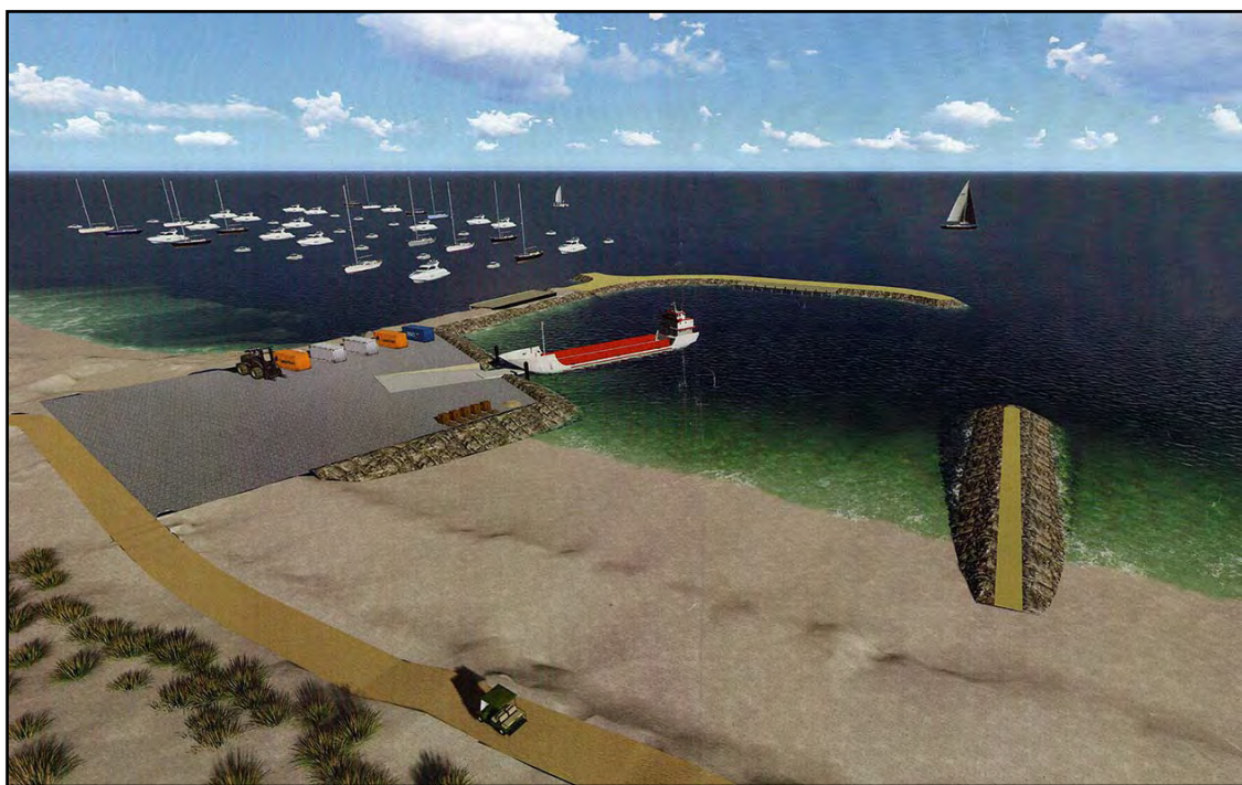
Figure 2: Rottneest Island Army Groyne – Proposed barge ramp and cargo handling facility Design Plan
