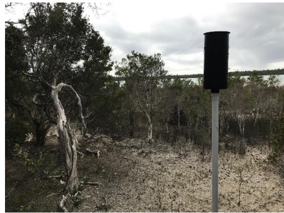
Figure 4: Location 2 Deposition Gauge
