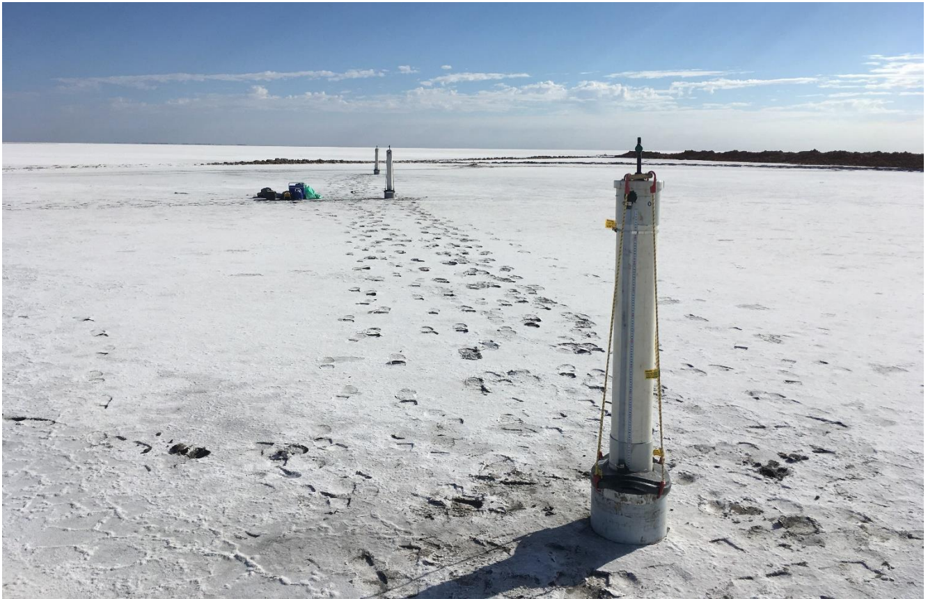
Figure 3. Operating constant head infiltration test.
