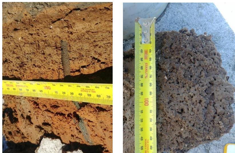
Figure 1: Pore structures observed in clay at infiltration test locations.
