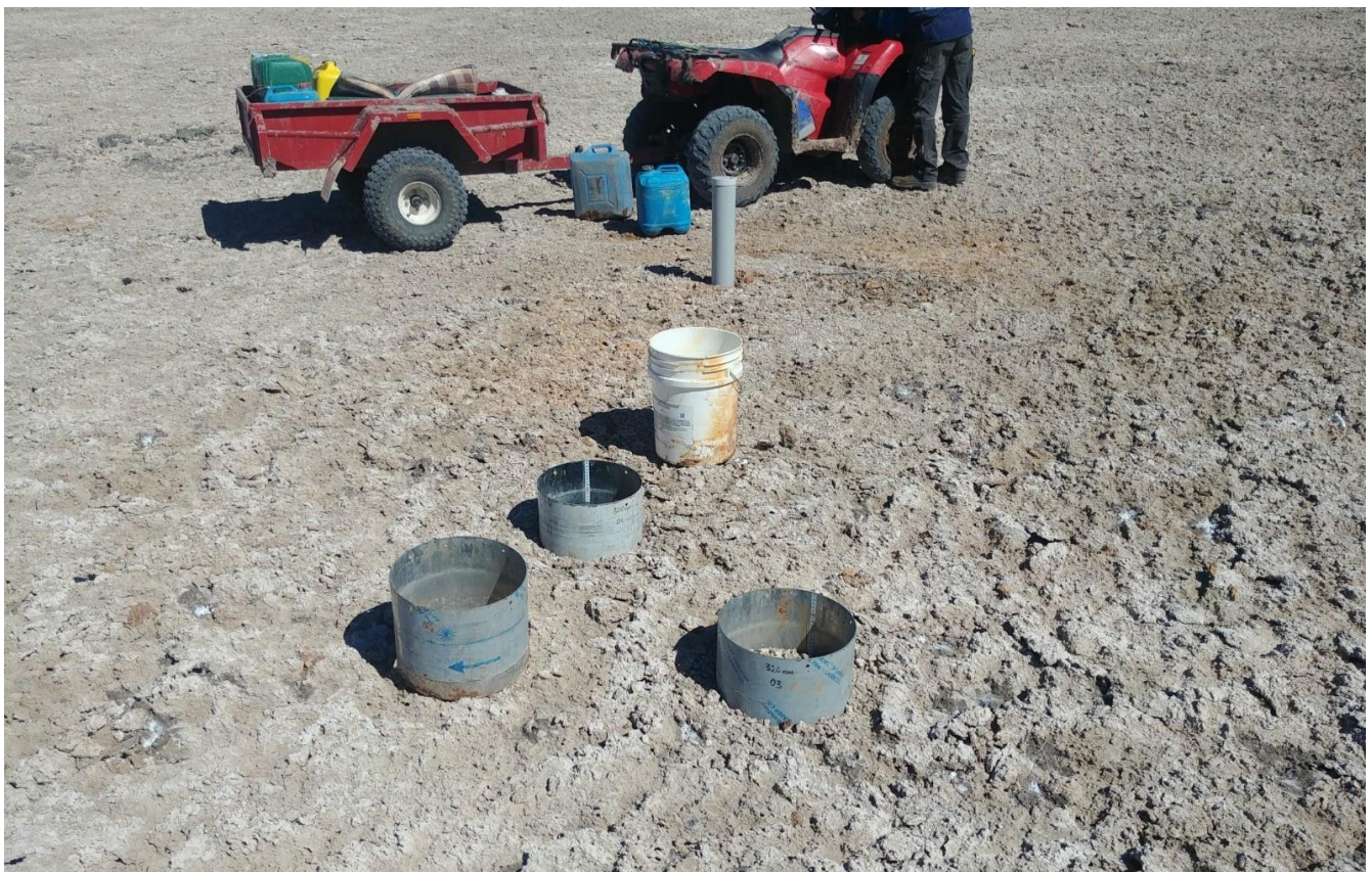
Figure 4. Falling head infiltration test equipment setup.
