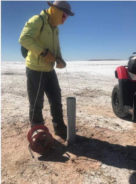
Figure 5. Pump out >2 bore volumes into a bucket until the turbidity is low.
