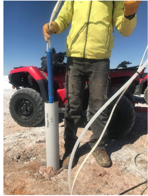
Figure 5. Pump out >2 bore volumes into a bucket until the turbidity is low.
