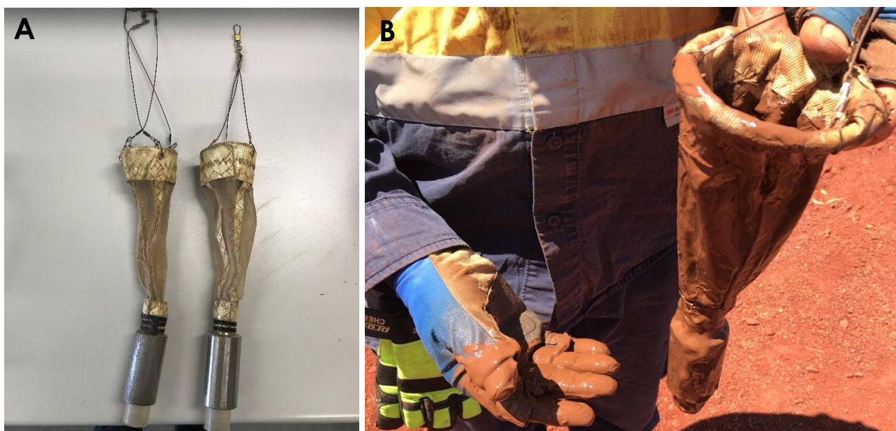
Plate 4-1: Examples of haul nets (A-B), used for sampling stygofauna.
