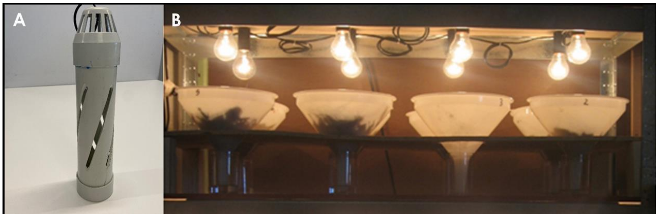
Plate 4-2: Troglofauna collection and extraction methods. (A) Litter trap, and (B) Tullgren funnels.
