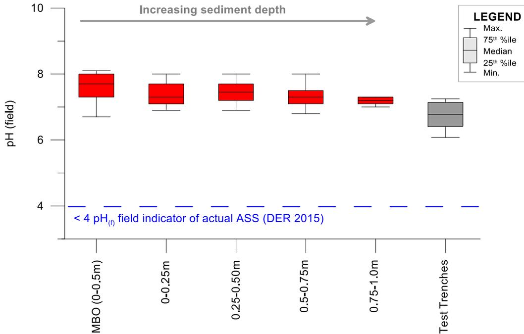
Figure 3 Field pH ( $pH_i$ ) with increasing sediment depth across all sites, including test trench water pH for reference
