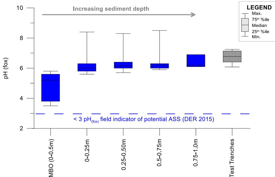
Figure 4 Chemically oxidised pH ( $pH_{fox}$ ) with increasing sediment depth across all sites, including test trench water pH for reference
