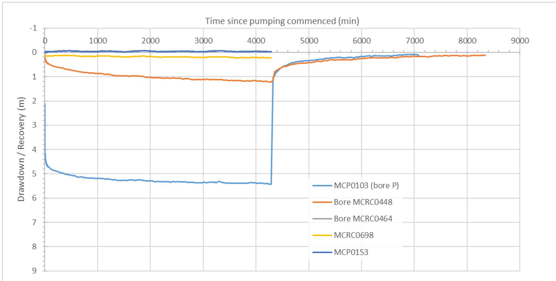
**Figure 7-3: Bore MCP0103 [P] aquifer response to pumping**
