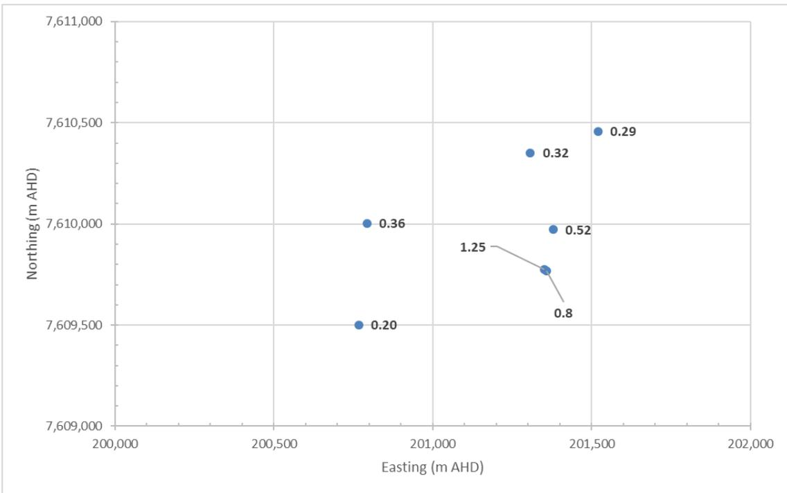
**Figure 7-12: MCP0152 [L] test - spatial response to pumping**
