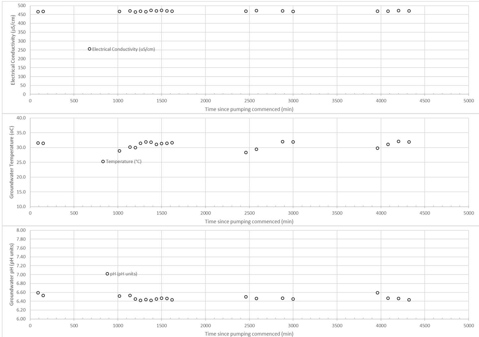
**Figure 7-17: MCP0153 [O] test - water quality monitoring**
