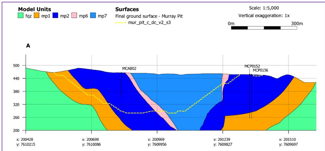
**Figure 8-2: Cross section 1: Murray Pit**
