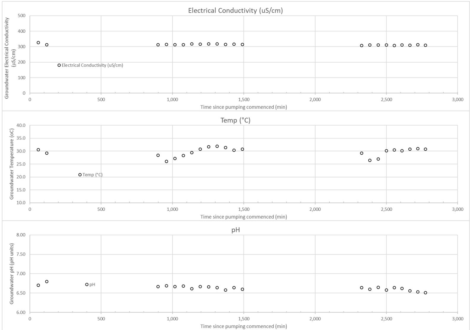
**Figure 7-9: MCP0151 [D] test - water quality monitoring**
