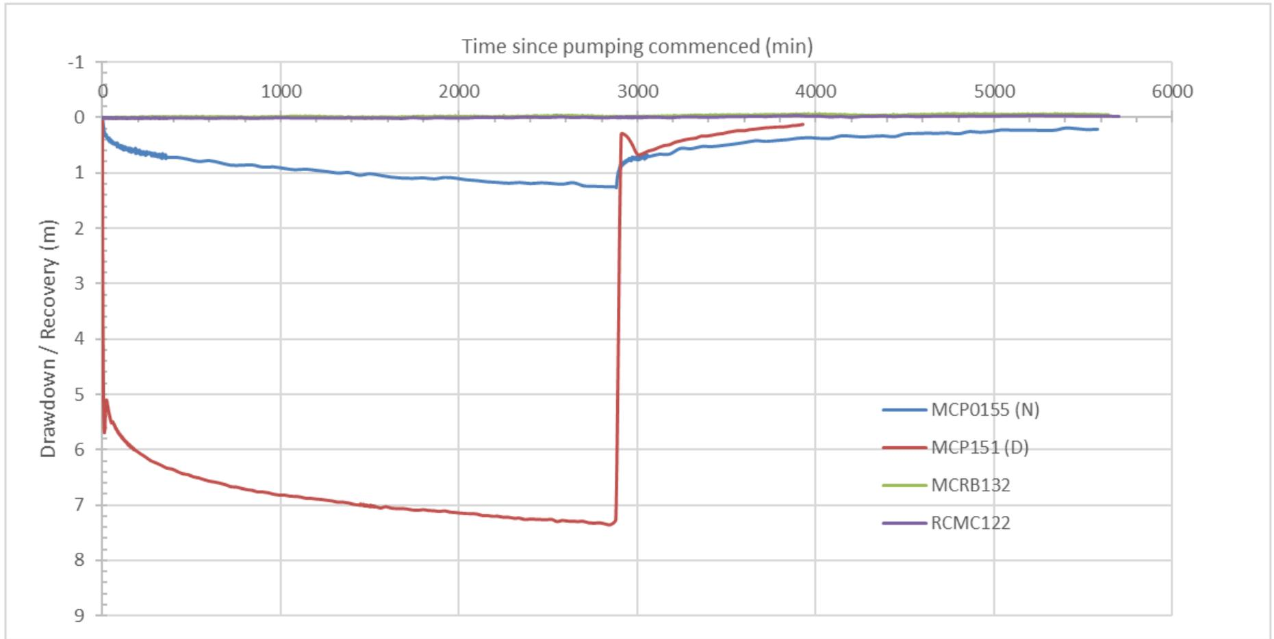
**Figure 7-8: MCP0151 [D] test - aquifer response to pumping**
