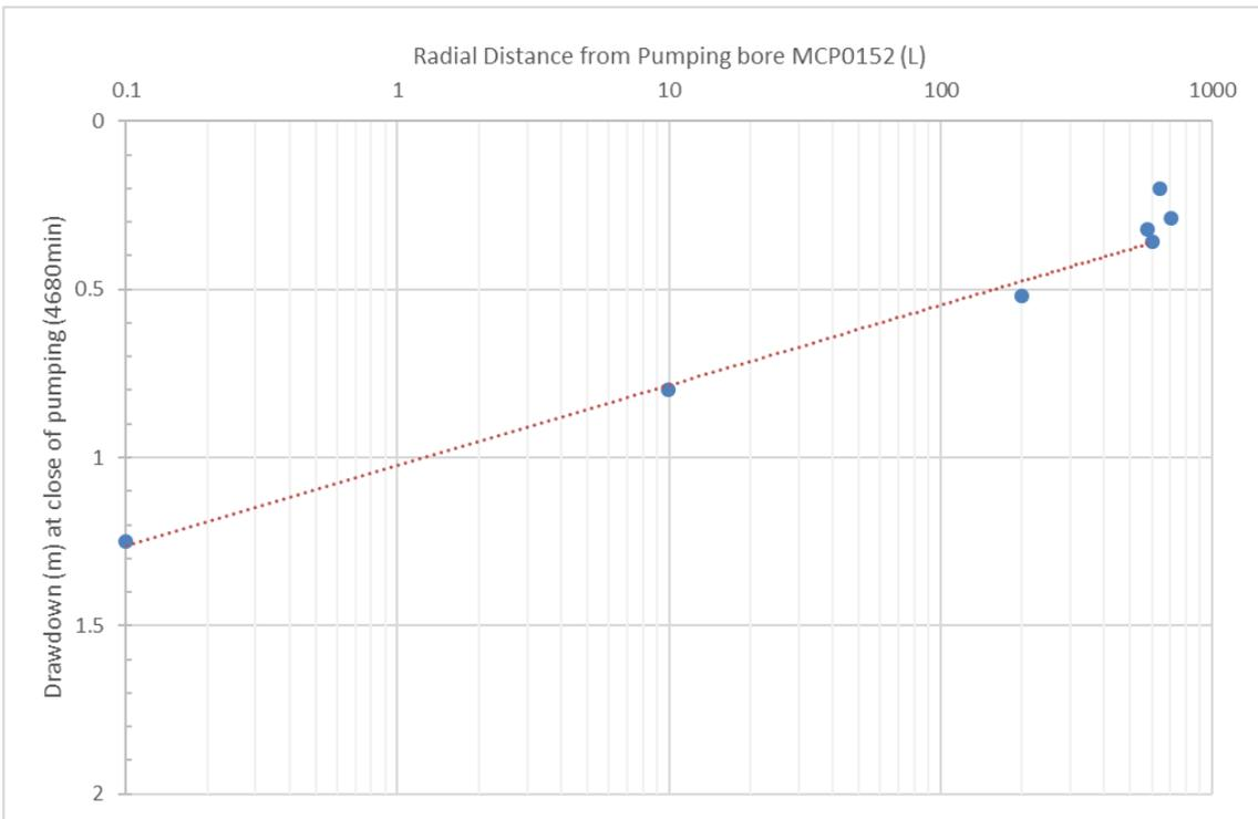
**Figure 7-13: MCP0152 [L] test - distance drawdown response**
