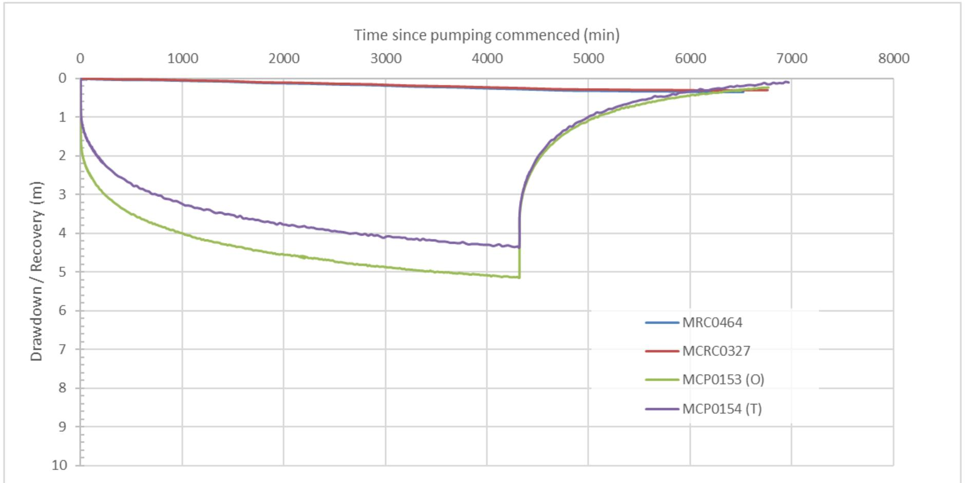
**Figure 7-16: MCP0153 [O] test - aquifer response to pumping**
