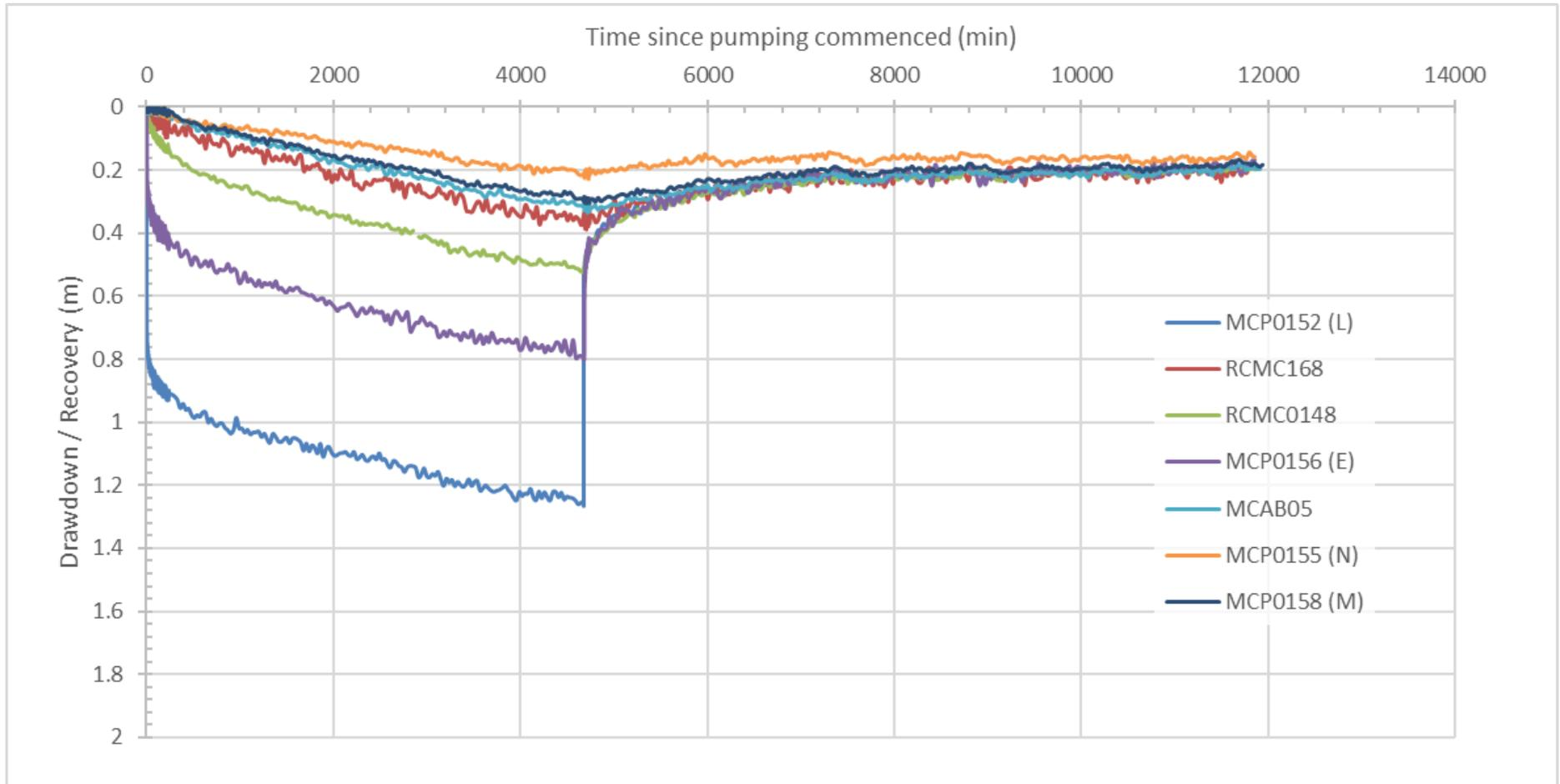
**Figure 7-11: MCP0152 [L] testing - aquifer response to pumping**
