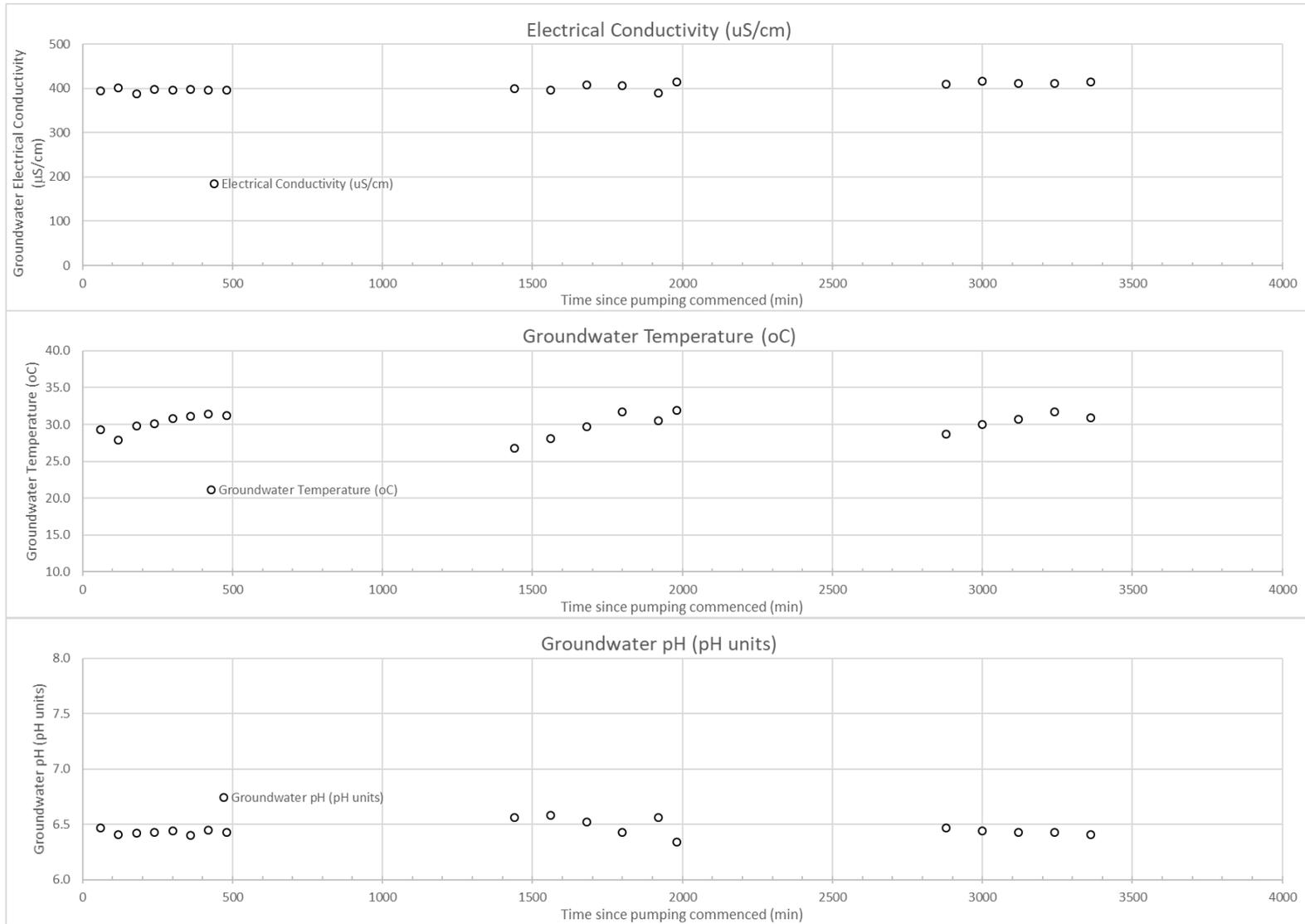
**Figure 7-14: MCP0152 [L] test - water quality monitoring**
