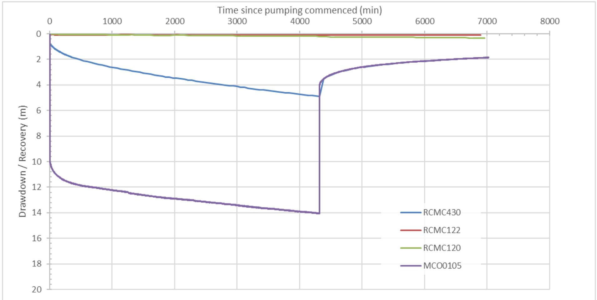
**Figure 7-5: MCP0105 [R] test response to pumping**
