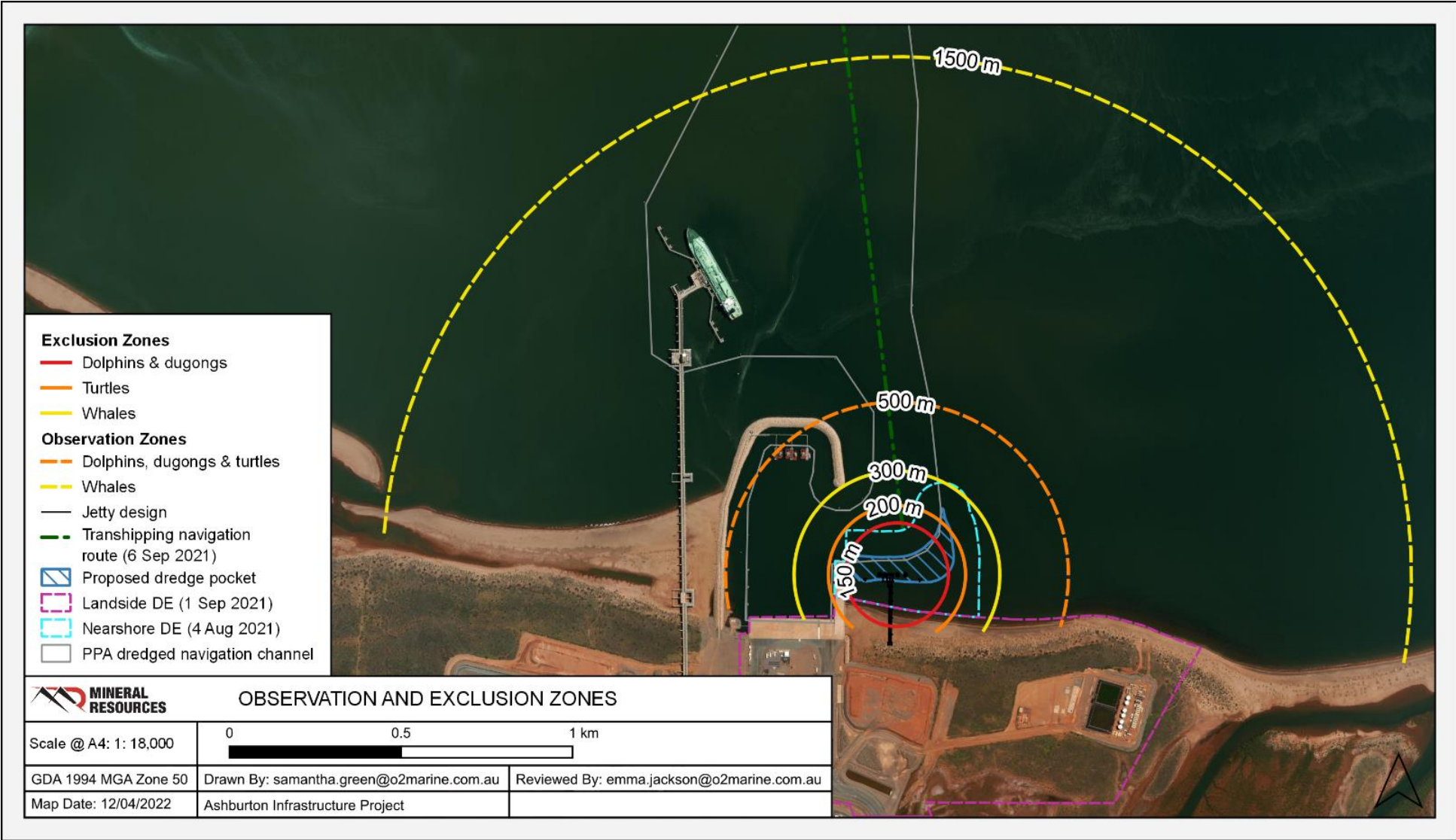
Figure 1 Marine Fauna Management Zones - Piling
