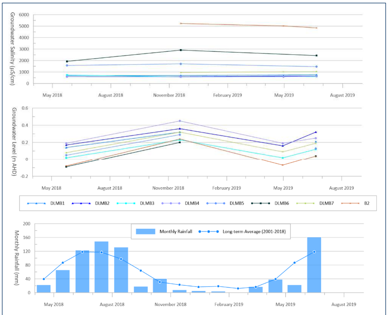
Figure 13: Groundwater Levels, Salinity and Rainfall (Monitoring Bores DLMB1-7)
