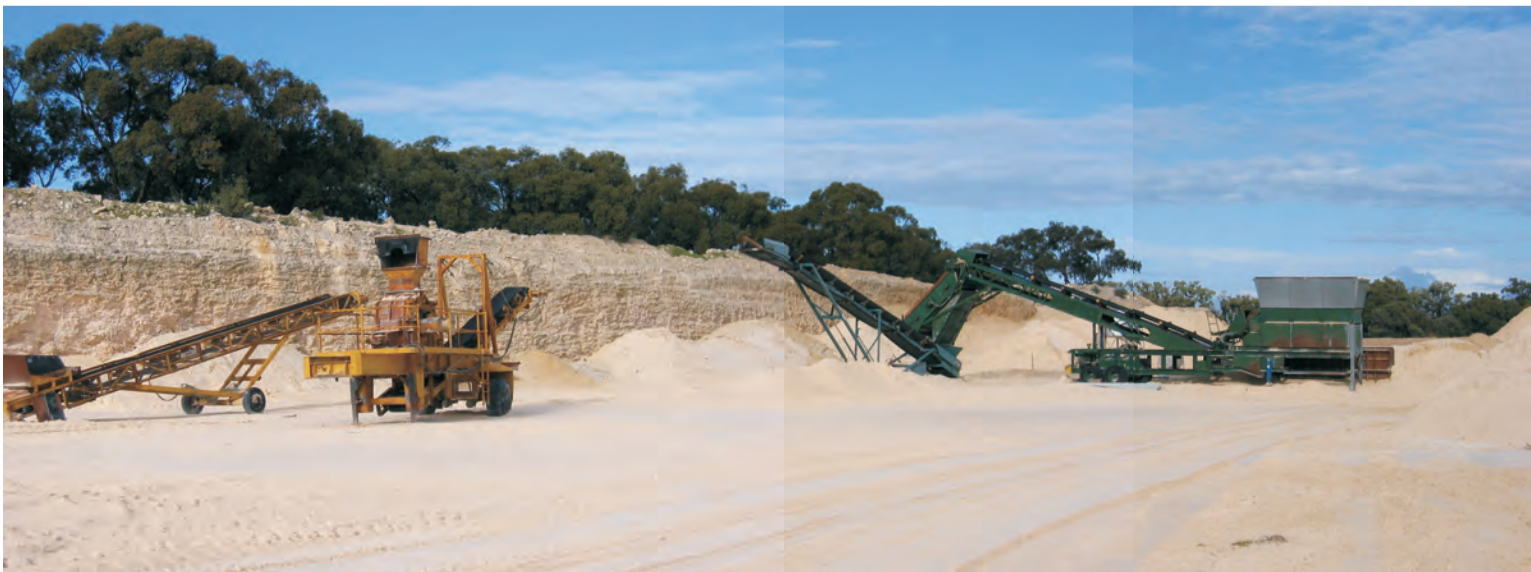
Processing at Myalup showing the face used for visual, noise and dust screening
