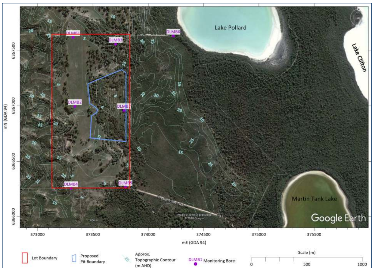
Figure 2: Site Topography and Monitoring Bore Locations
