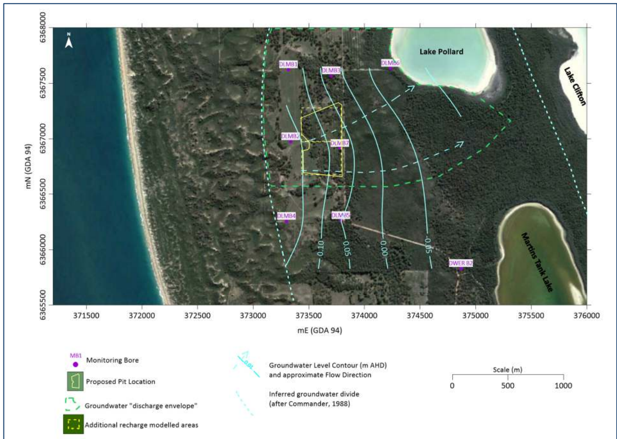
Figure 21: Approximate Area Providing Groundwater Discharge to Lake Pollard
