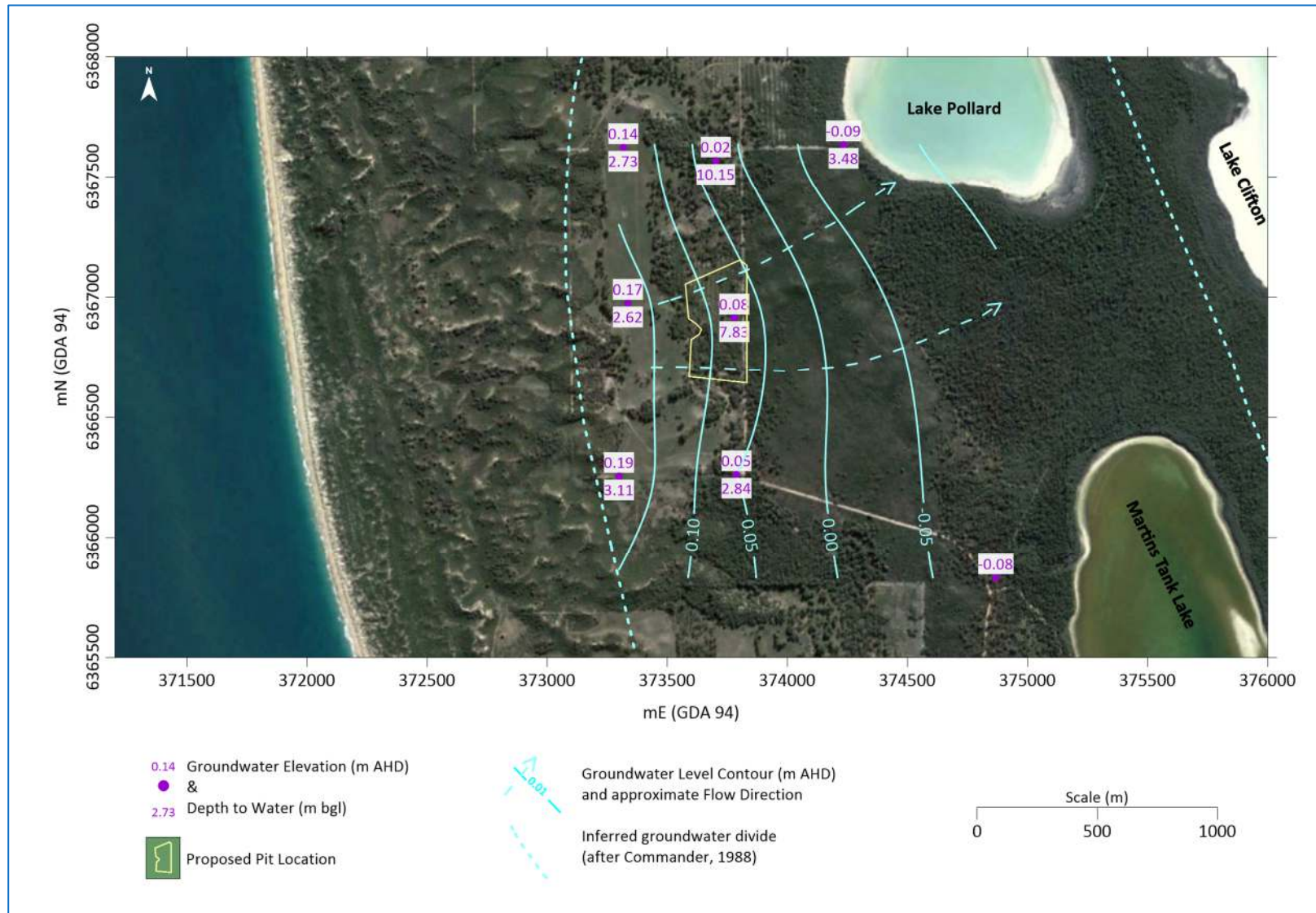
Figure 12: Groundwater Level Contours – 24 May 2018
