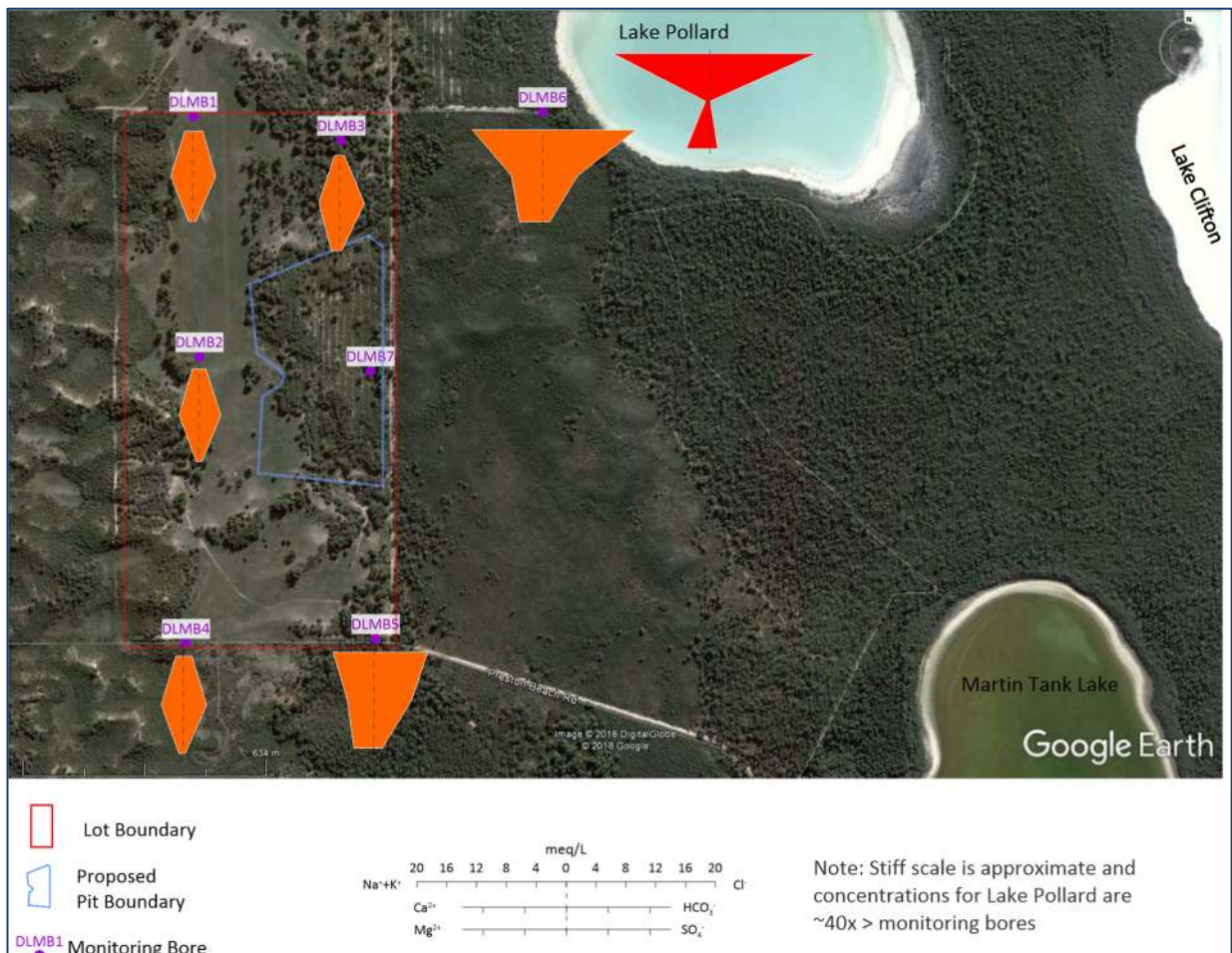
Figure 17 - Stiff Diagrams for 2018 Sampling Results Showing Spatial Trends for Groundwater Composition
