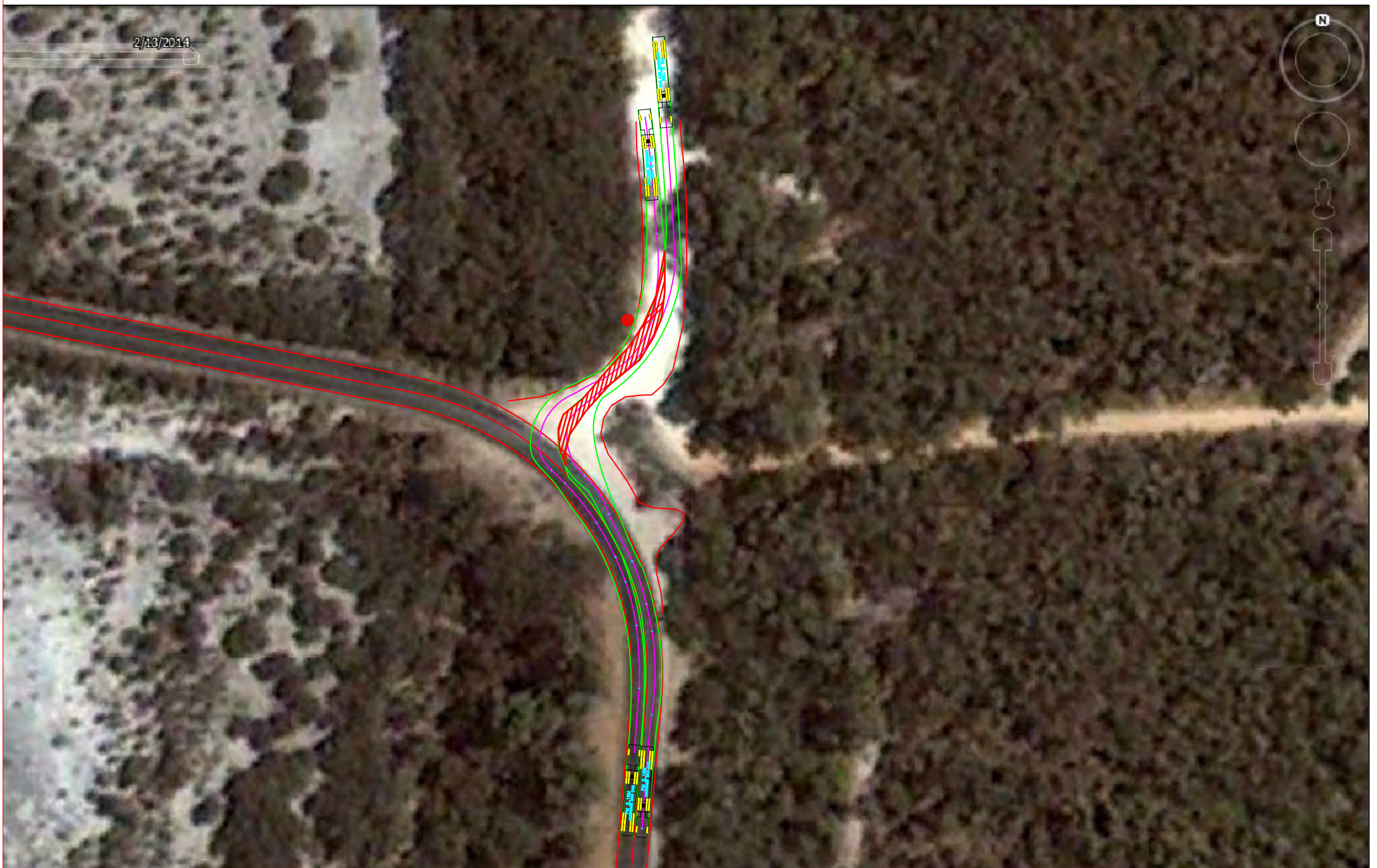
DESIGN VEHICLE 19M SEMI-TRAILER PLAN SHOWING CONFLICT BETWEEN 19M SEMI'S TURNING-IN AND TURNING-OUT
