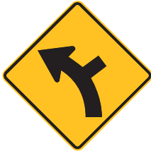
SIDE ROAD JUNCTION ON A CURVE
