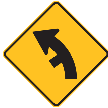
SIDE ROAD JUNCTION ON A CURVE
