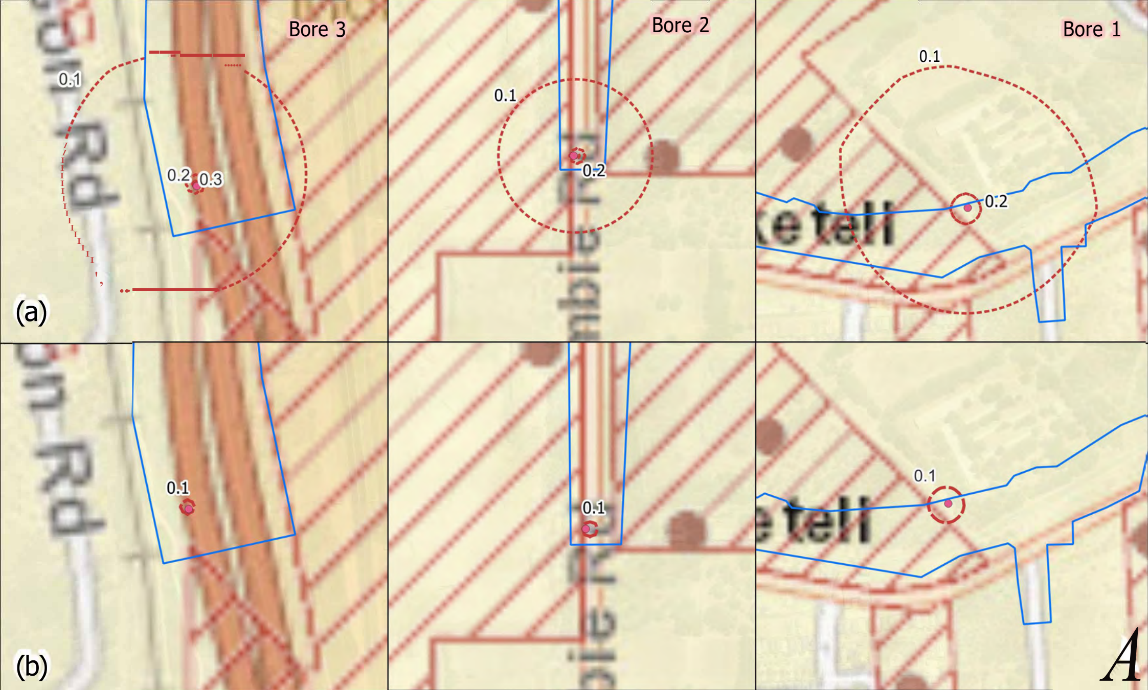
Figure 17: Current SC groundwater licences with drawdown from {a} Scenario 3a {b} Scenario 3b
