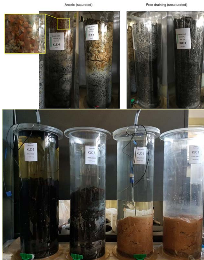
Figure 5-1: Example of large kinetic leach column (KLC) tests operated as ‘free-leach’ and saturated.
