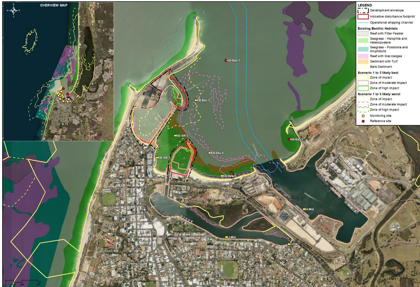
Figure 8: Water quality monitoring locations during for the probable, serial and parallel construction sequences
