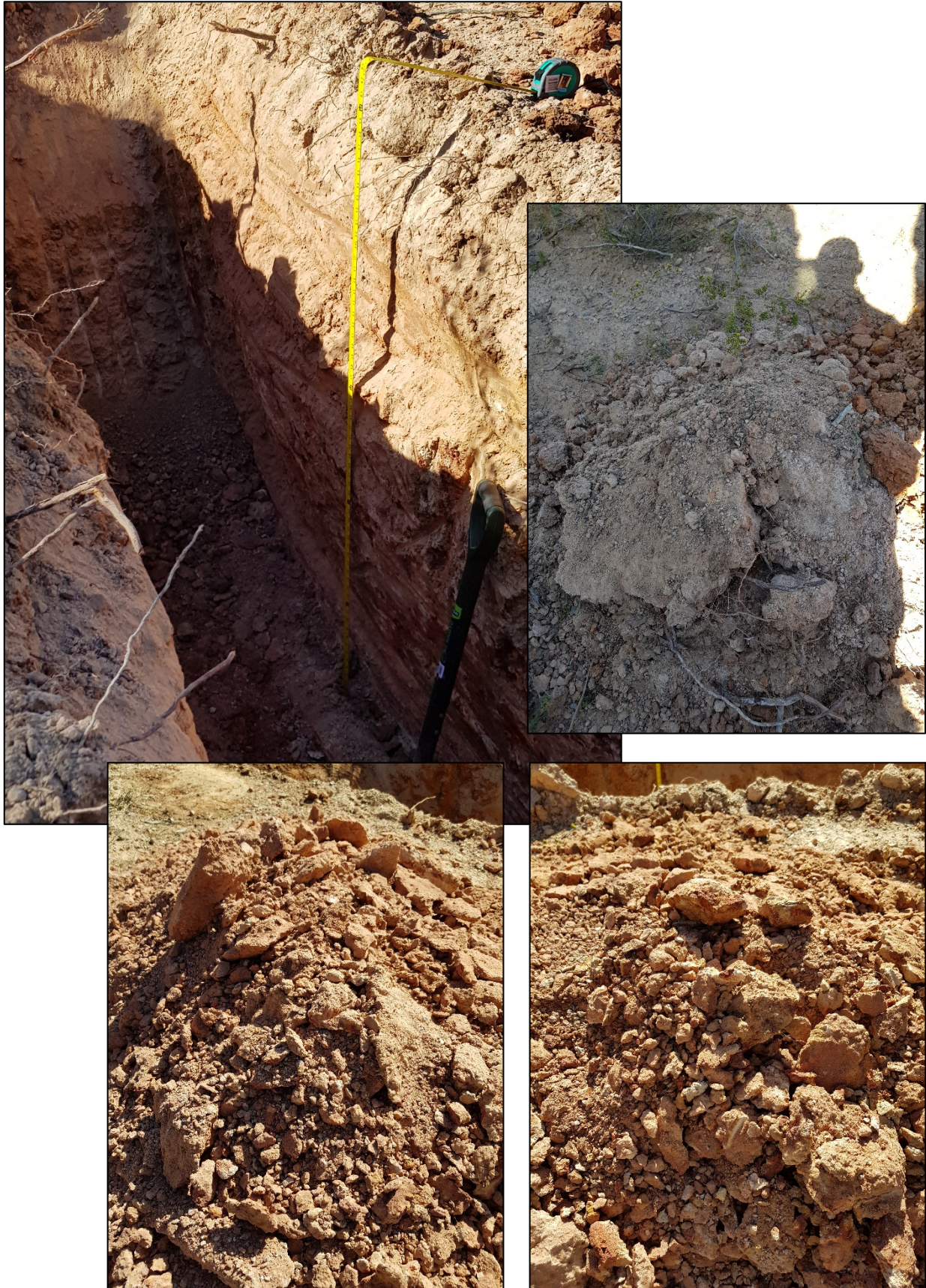
Test pit TP 01 – 1.6m to refusal, 3 soil horizons in a clockwise rotation starting top right; TOPSOIL, ALLUVIUM (red brown sandy silt) and ALLUVIUM (white mottled sandy silt).
