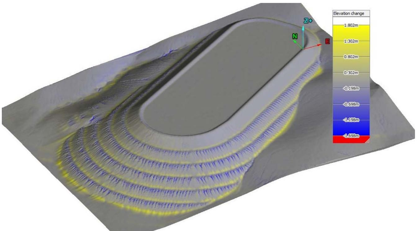
South WRL modelled erosion with topsoil layer and 30% cover
