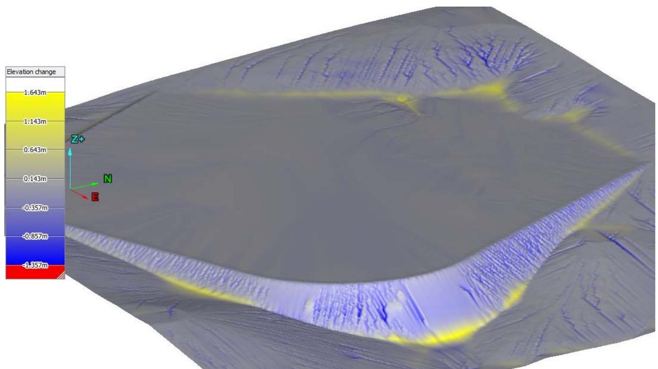
TSF modelled erosion with topsoil and fresh rock layer (50:50 mix) and 70% cover
