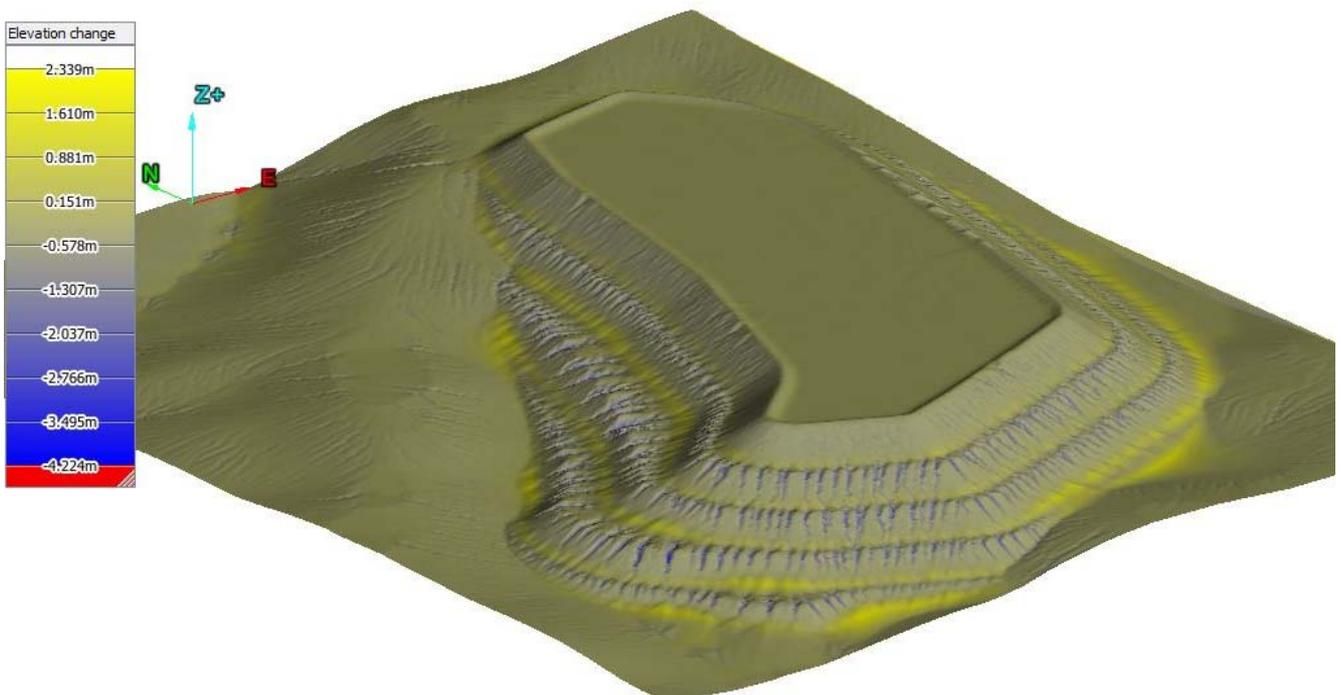
South WRL modelled erosion with topsoil and fresh rock layer (50:50 mix) and 70% cover
