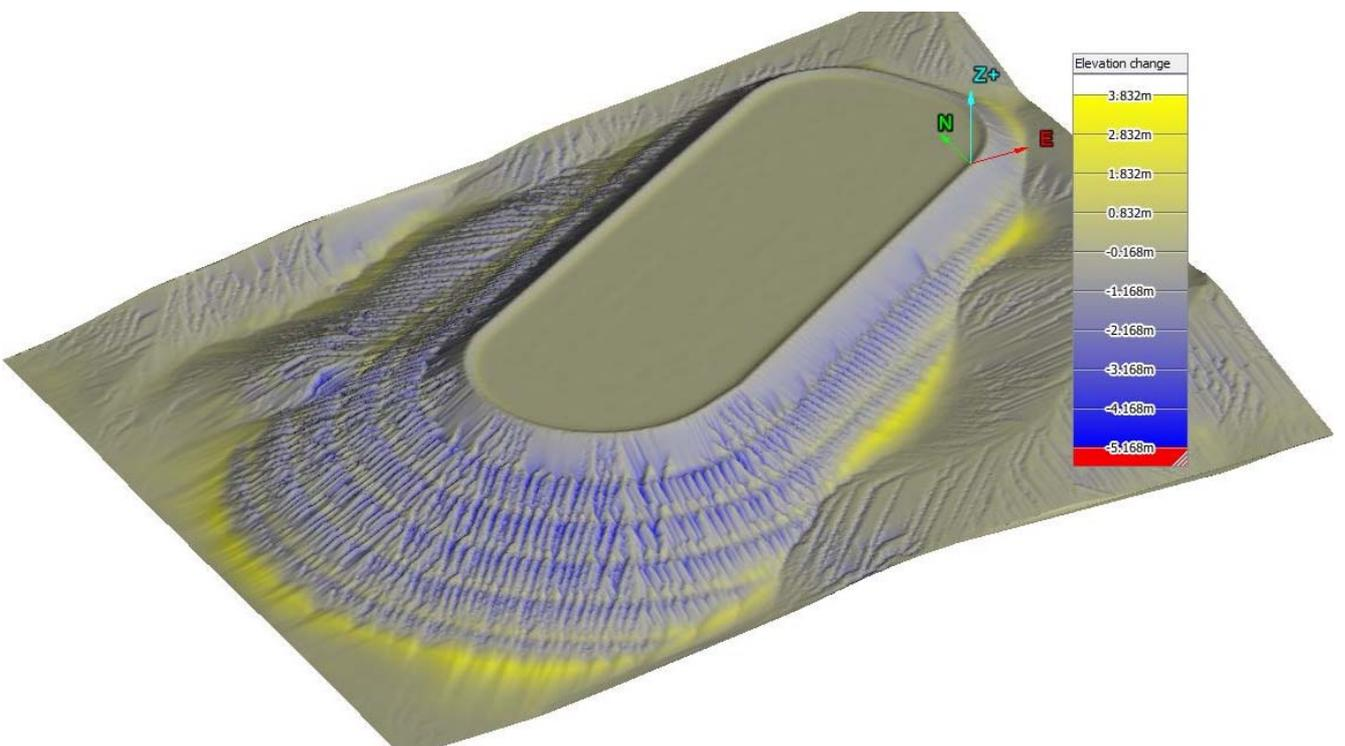
North WRL modelled erosion with topsoil layer and 70% cover
