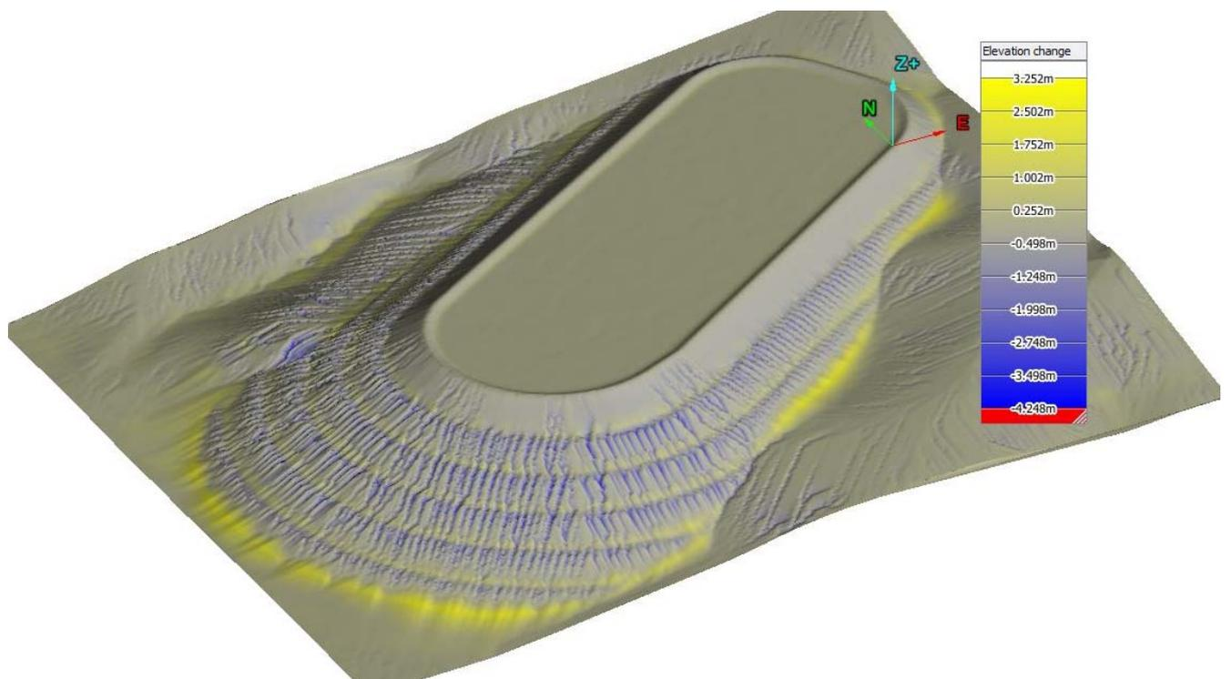
North WRL modelled erosion with topsoil and fresh rock layer (50:50 mix) and 30% cover
