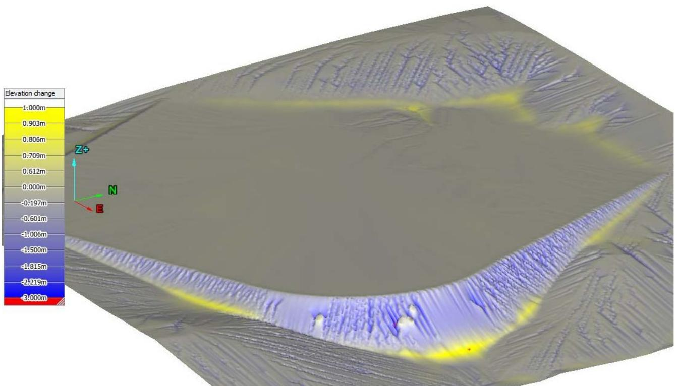
**TSF modelled erosion with topsoil layer and 70% cover**
