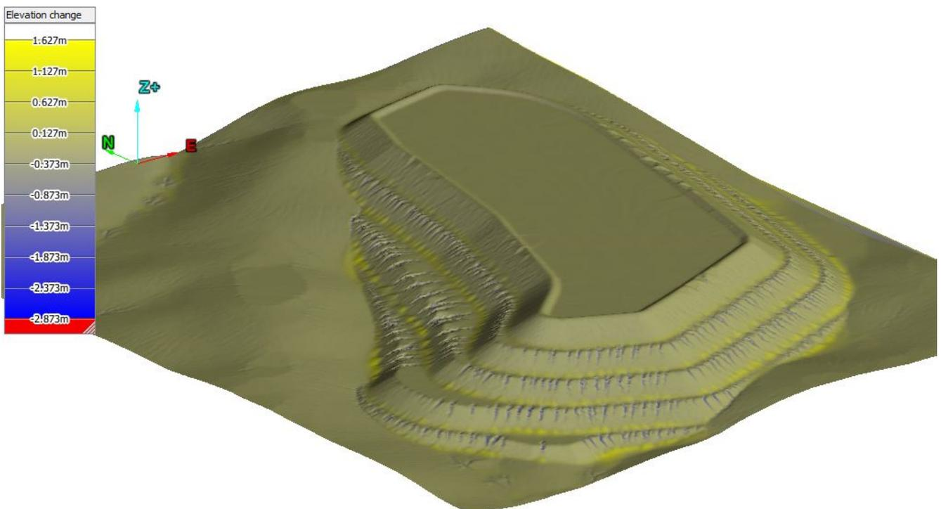
**TSF modelled erosion with topsoil layer and 30% cover**
