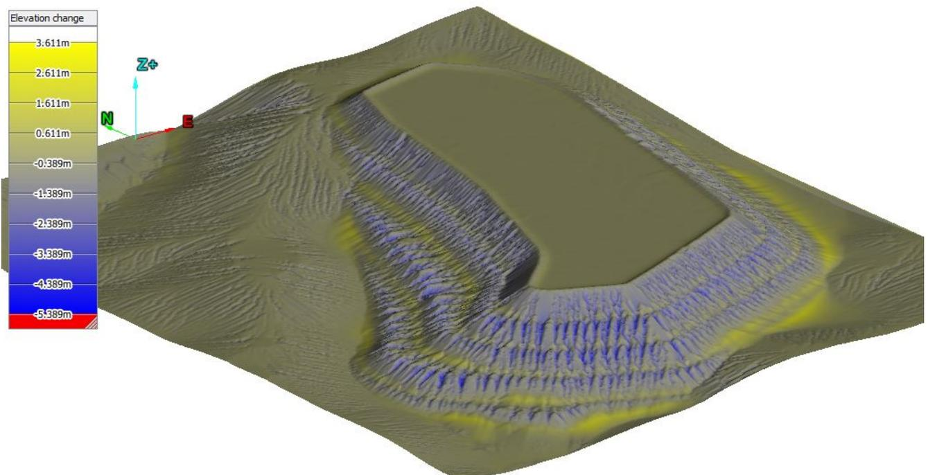
South WRL modelled erosion with topsoil layer and 70% cover
