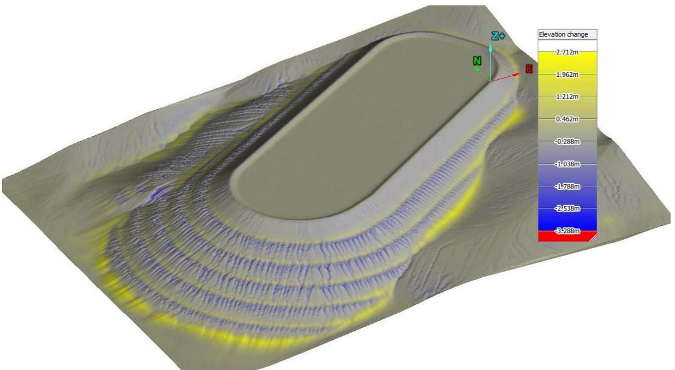
North WRL modelled erosion with topsoil and fresh rock layer (50:50 mix) and 70% cover
