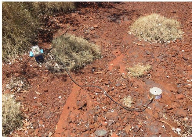
A geophone glued to rock mass, ready to capture blast vibration data
