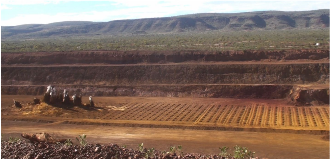
Production blast at Hope Downs 1 mine
