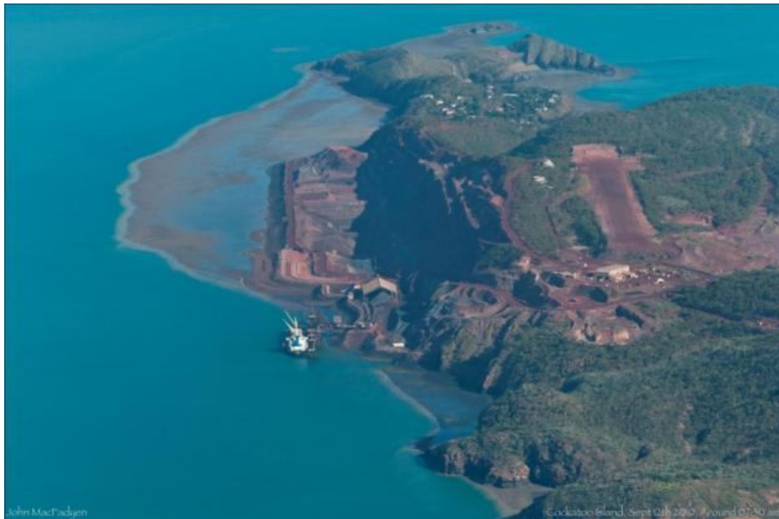
Figure 3. Cockatoo Island in September 2010, looking west. Image shows the High Wall, Pit, Seawall and reef flat exposed at a spring low tide. Image courtesy of John McFadyen.
