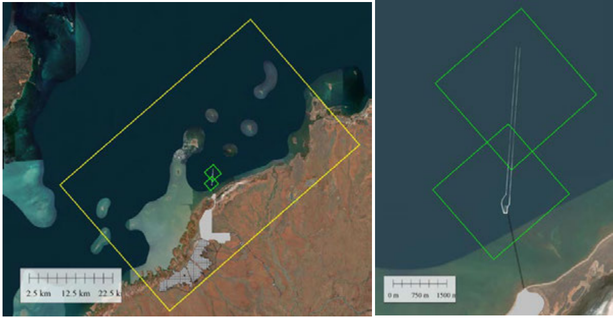
Figure 4.2: Local Delft3D Hydrodynamic Model grid setup applied for dredge plume modelling. Domain Decomposition Grids - Outer grid (yellow, grid resolution 200m x 200m) and Inner grids (green, grid resolution 40m x 40m).
