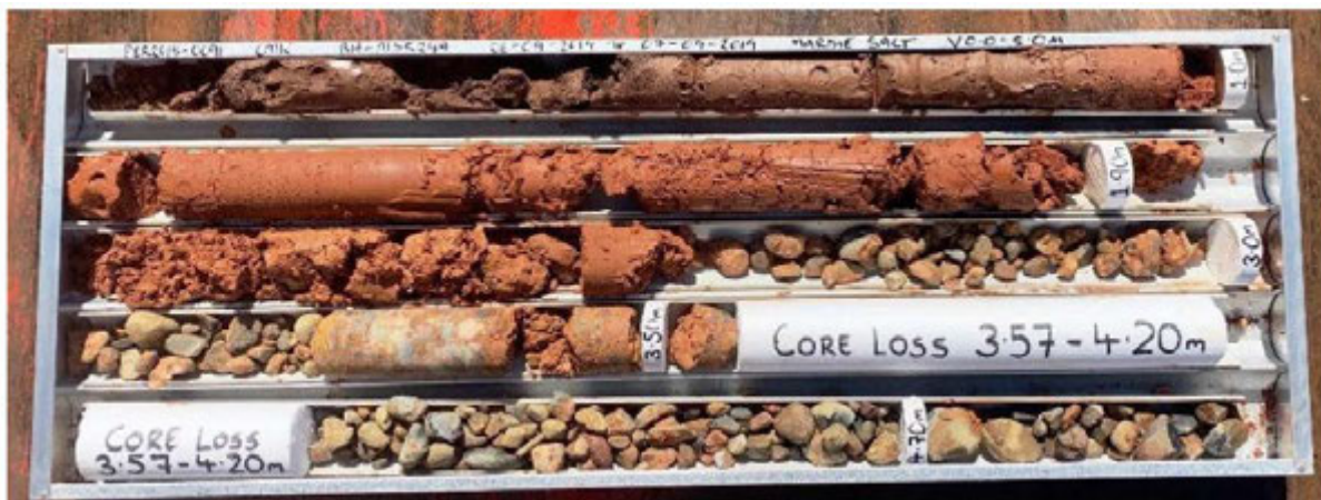
Figure 3.5: Core Sample for site MS529-A (TAMS, 2019). Cores at 1m length are shown as recovered from the seabed. Sediment sampling from the core was extracted from 1.2m – 1.35m below the surface and showed very high fines content of 82% (CMW, 2019).
