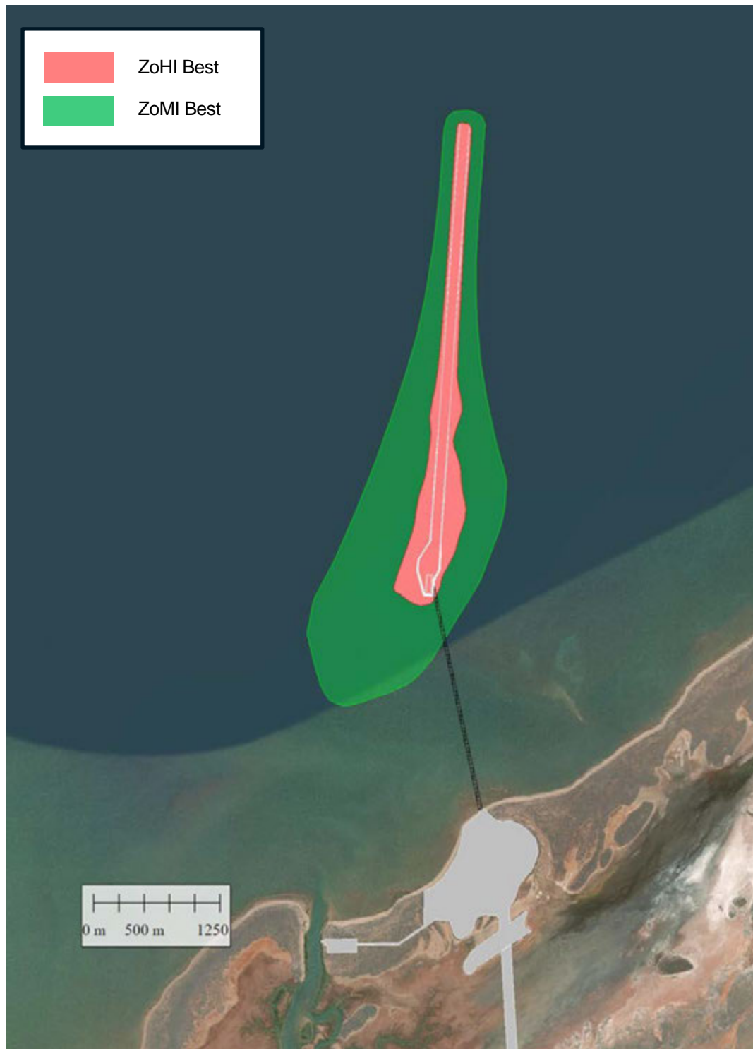
Figure 5.11: Calculated Zones of Impact for expected production rate scenario with a dredging rate of 2,000m 3 /day ('Best Case'). Full dredge program.
