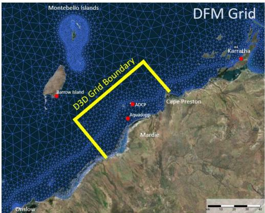
Figure 4.1: Upper plot – Regional Hydrodynamic Model Domain (DFM). Lower plot – Local scale Delft3D model developed for Mardie Project with boundary conditions defined from the Regional model. Measured data was available for model validation from the ADCP and Aquadopp Locations.
