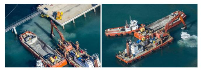
Figure 6. Example of a Backhoe Dredge proposed for Project dredging.
