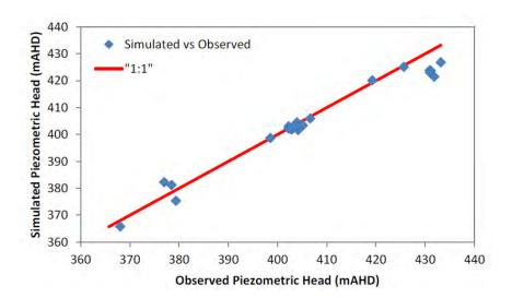
Figure 2-2 Observed versus modelled water levels for steady state calibration
