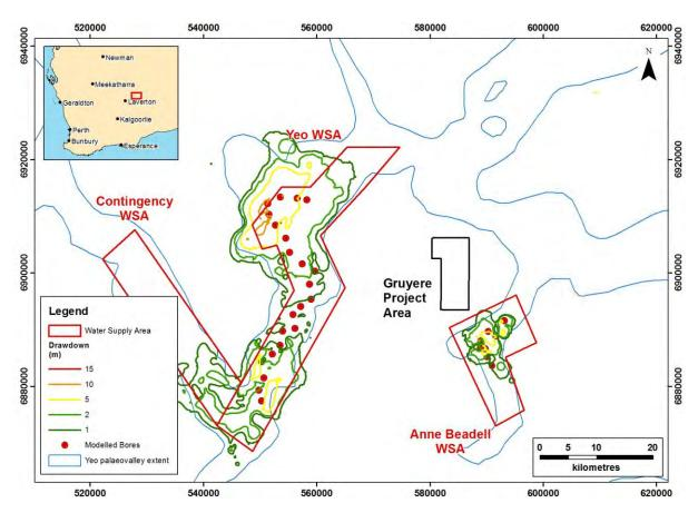
Figure 3-1 Modelled drawdown at year 15 (end of mining) for the Quaternary Alluvial and Calcrete Aquifer (Slice 2)
