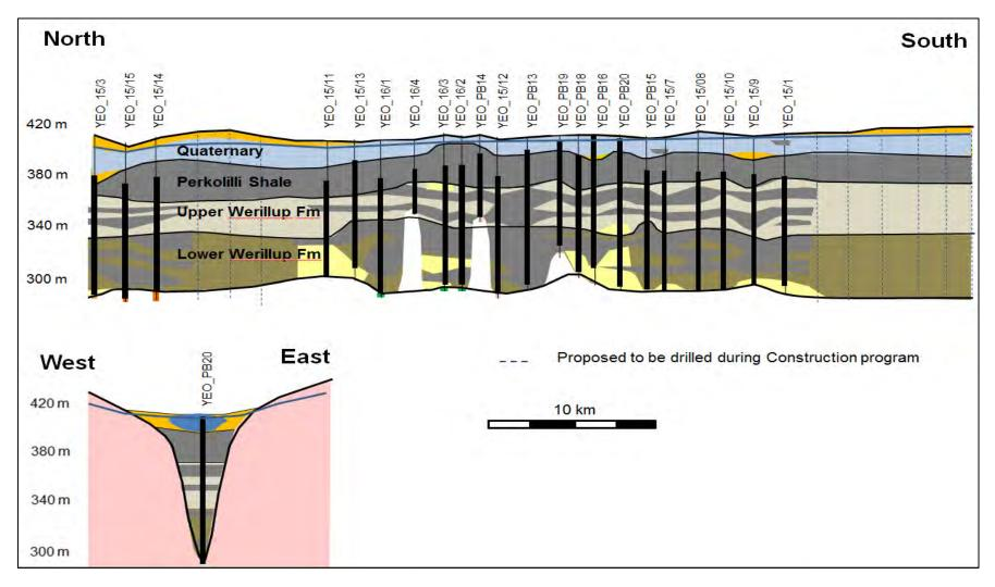
Figure 5: Geological Long and Cross Section through the Yeo Borefield
