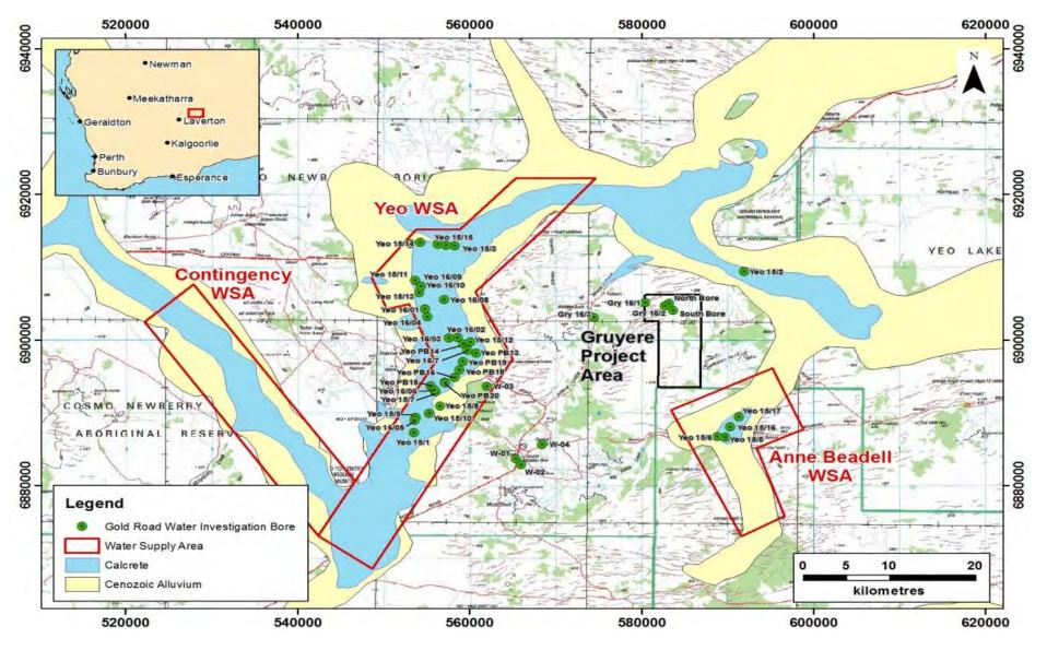
Figure 7: Extent of the Alluvial Valley and Near Surface Calcrete over the Yeo Borefield
