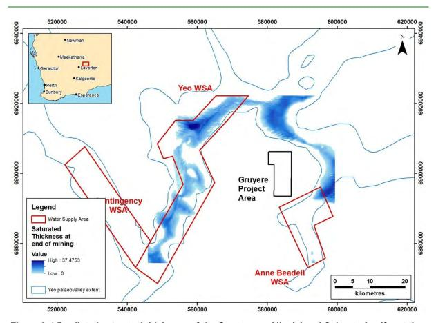
Figure 3-4 Predicted saturated thickness of the Quaternary Alluvial and Calcrete Aquifer at the end of mining
