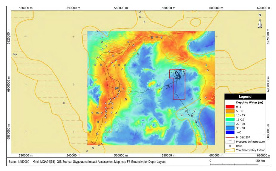
Figure 8: Depth to Groundwater within the Yeo Palaeochannel
