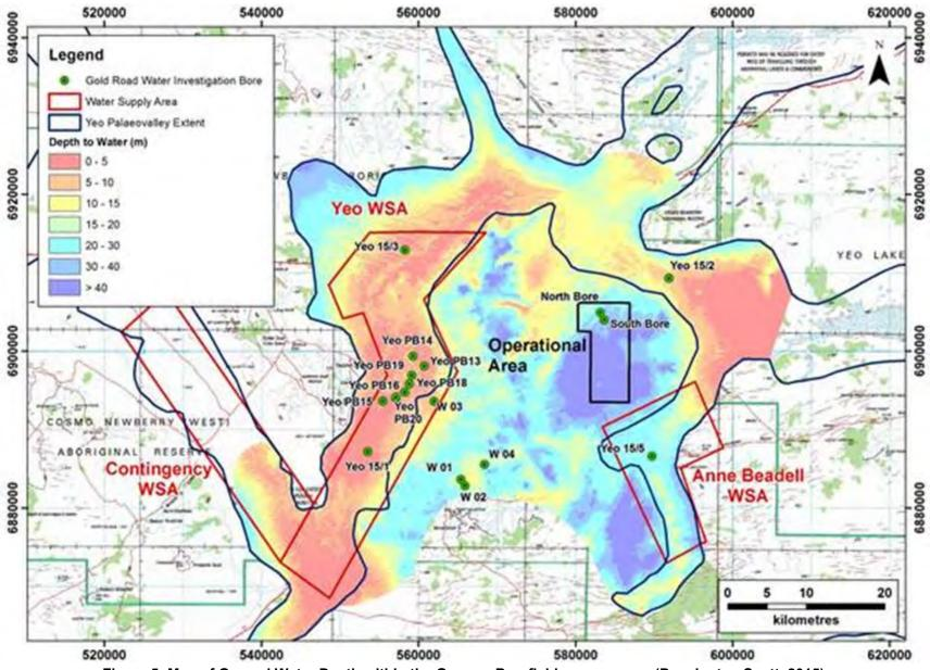
Figure 5: Map of Ground Water Depth within the Gruyere Borefields survey area (Pennington Scott, 2015)
