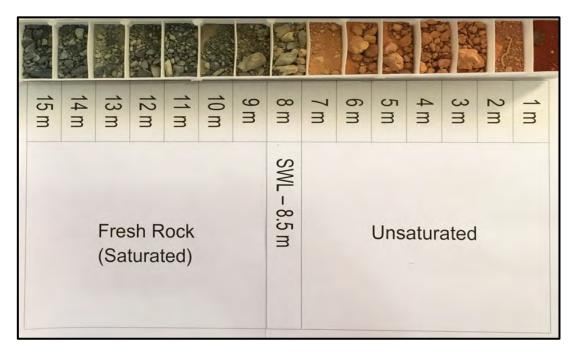
Plate 2: Bore Log for Bore 16GYWB0016
