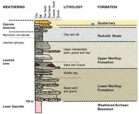
Figure 4. Profile through the Yeo Palaeochannel (from Pennington Scott 2016).
