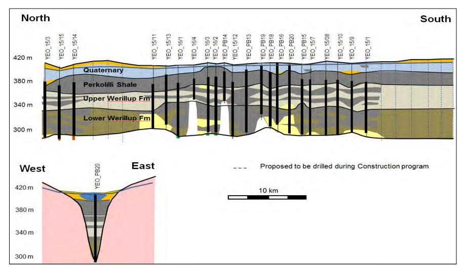
Figure 9: Geological Long and Cross Section through the Yeo Borefield
