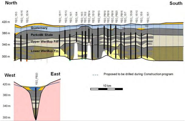
**Figure 5.** Longitudinal and cross section of the Yeo Palaeochannel. (From Pennington Scott 2016).
