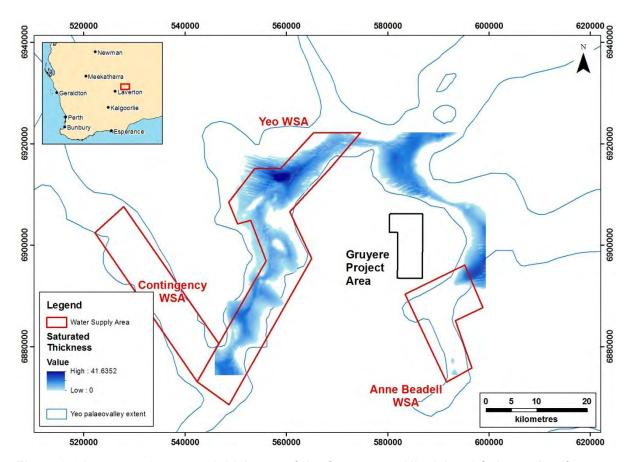
Figure 3-3 Interpreted saturated thickness of the Quaternary Alluvial and Calcrete Aquifer
