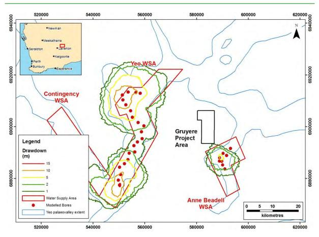
Figure 3-2 Modelled drawdown at year 15 (end of mining) for the Werillup Formation (Slice 5)
