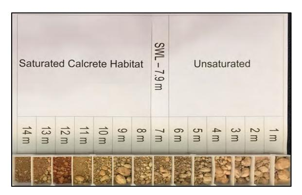
Plate 3: Bore Log for Bore 16GYWB0025
