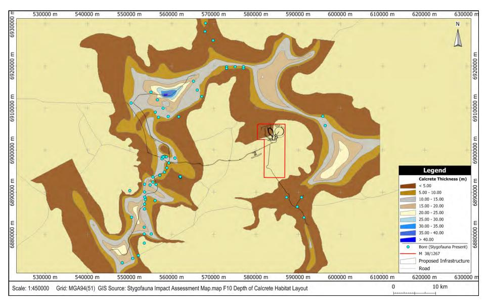
Figure 10: Depth of the Calcrete Extent (Saturated and Unsaturated) of the Yeo Palaeochannel
