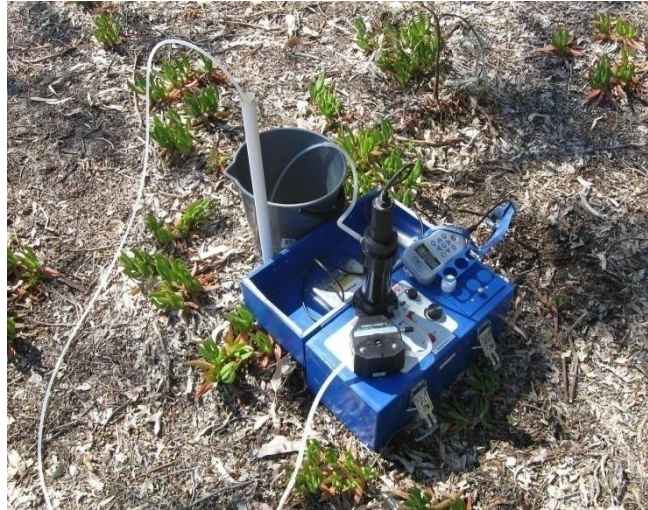
Figure 5 Sampling set up of the 25 mm piezometer
