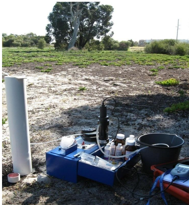
Figure 6 Sampling set up of the 50 mm piezometer
