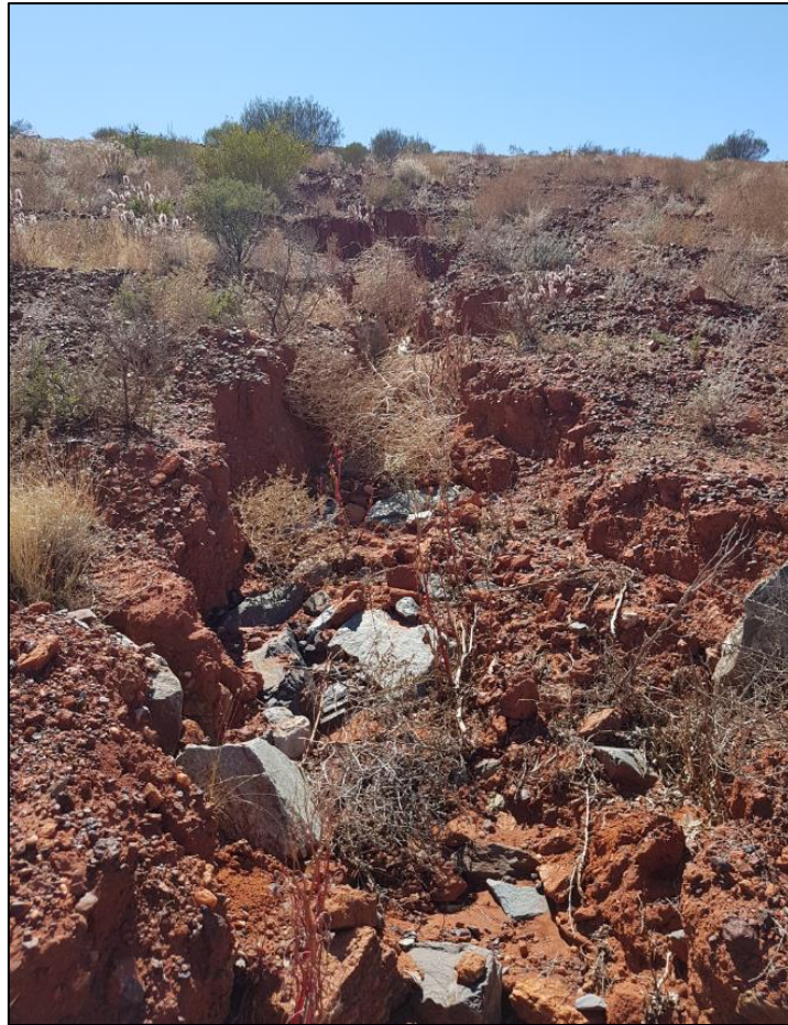
Plate 7-1: Erosion Gullies Observed in Concave Slope Trials
