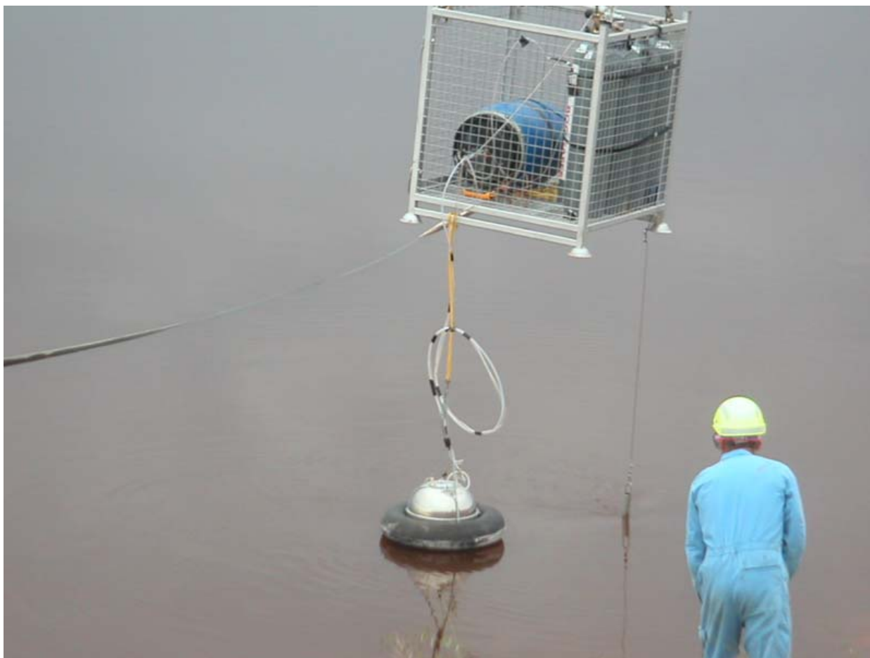
Figure 3. Sampling hood connected to Automated Sampling system
