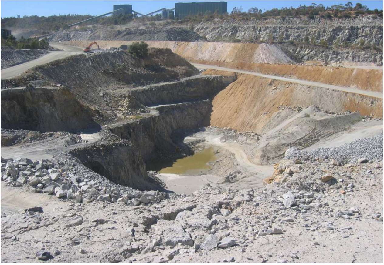
Plate 5: Present Red Hill Quarry showing workings approximately 100m deep, probably below regional groundwater table.
