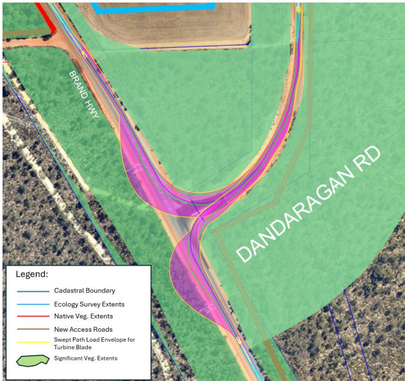
Figure 7-2: Dandaragan Road/ Brand Highway swept path analysis
