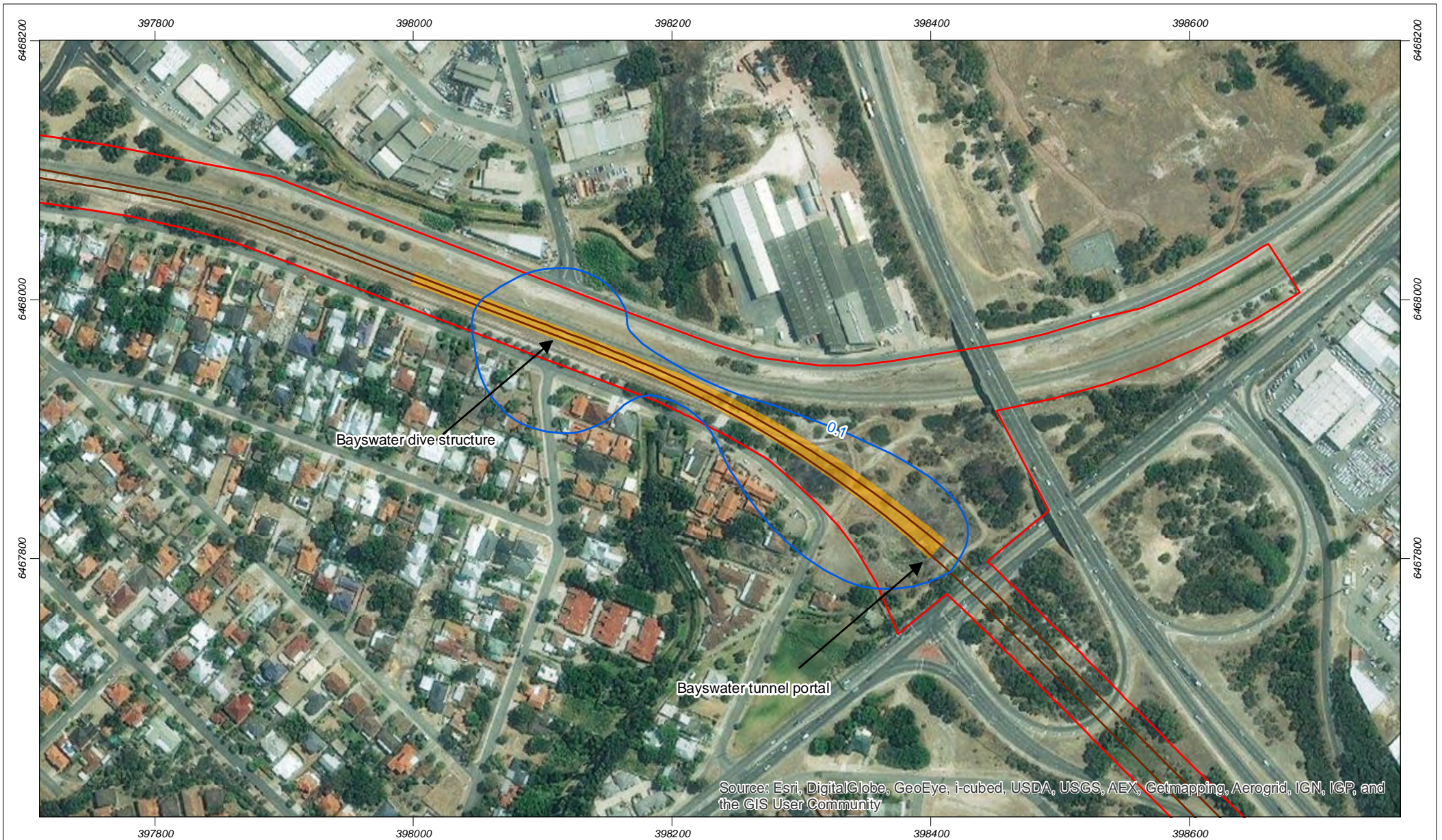
Figure 5-1: Groundwater drawdown contours for Bayswater tunnel portal and dive structure after 16 weeks
