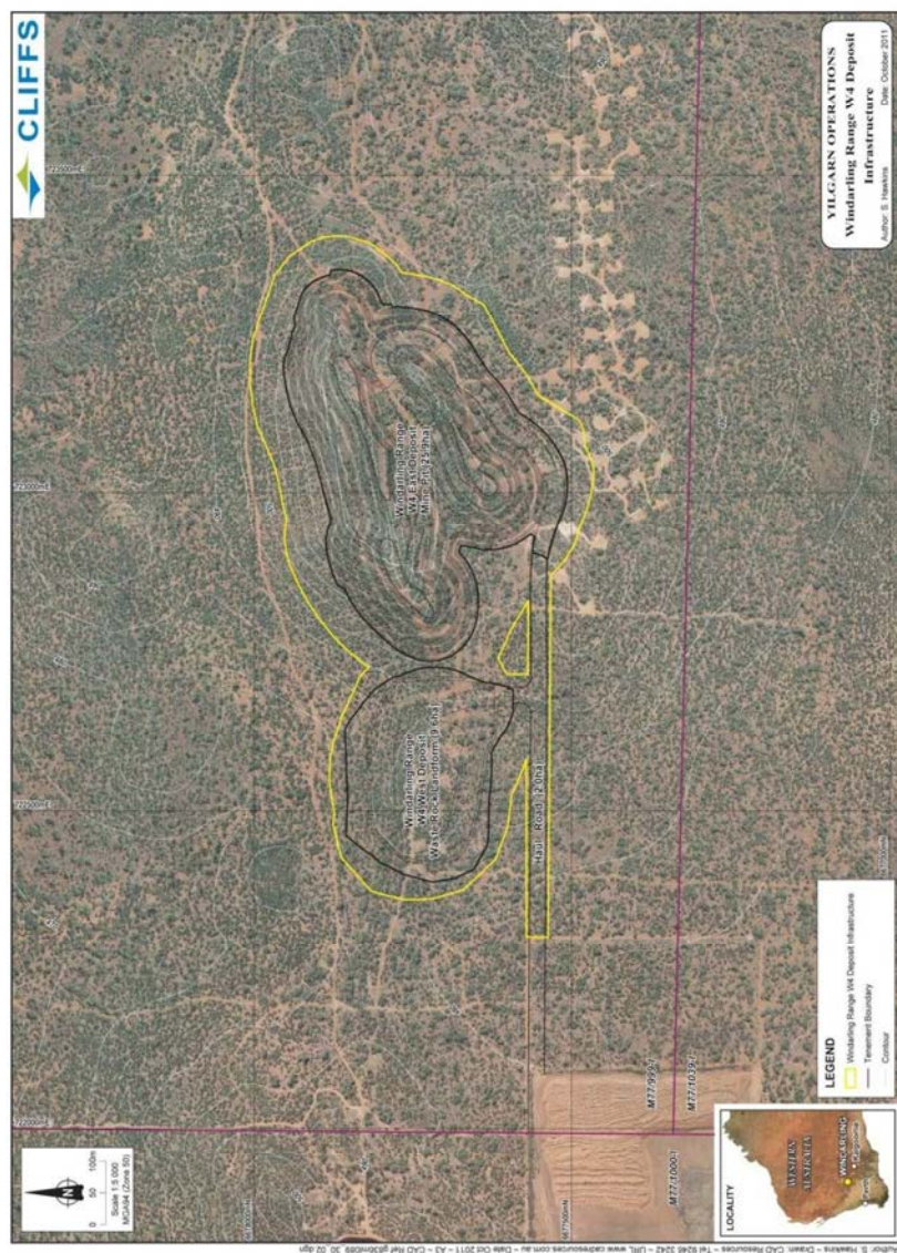
Figure 2-3 Layout of the Windarling Range W4 Deposit Infrastructure. The Windarling Range W4 Deposit infrastructure comprises of the Windarling Range W4 West Deposit Mine Pit, Windarling Range W4 East Deposit Mine Pit, Windarling Range W4 West Deposit Waste Rock Landform and the Windarling Range W4 Deposit Haul Road. For image clarity, the Windarling Range W4 West Deposit Mine Pit is not shown as it coincides with the same area of the Windarling Range W4 West Deposit Waste Rock Landform.
