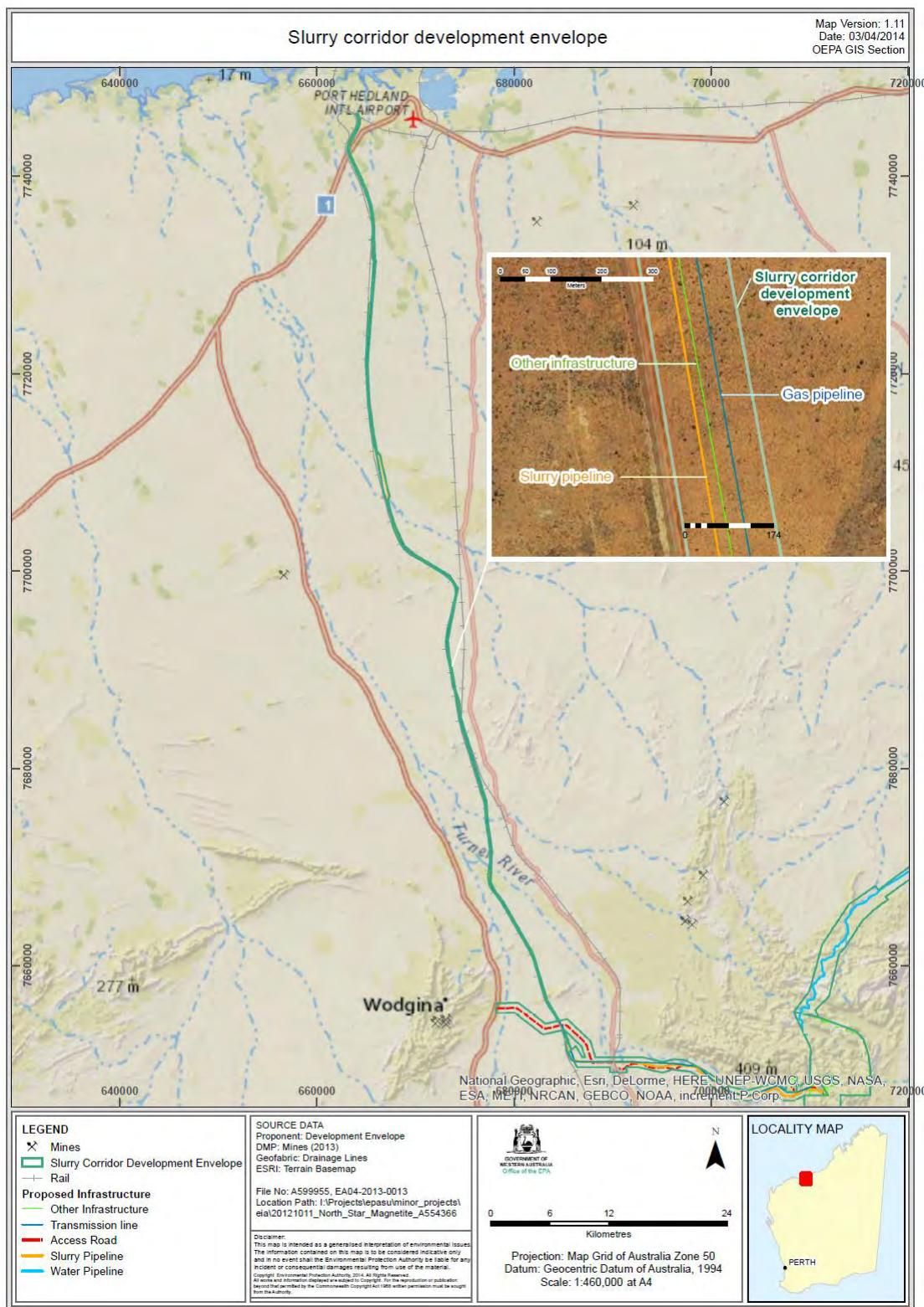
**Figure 3 Slurry corridor development envelope**
