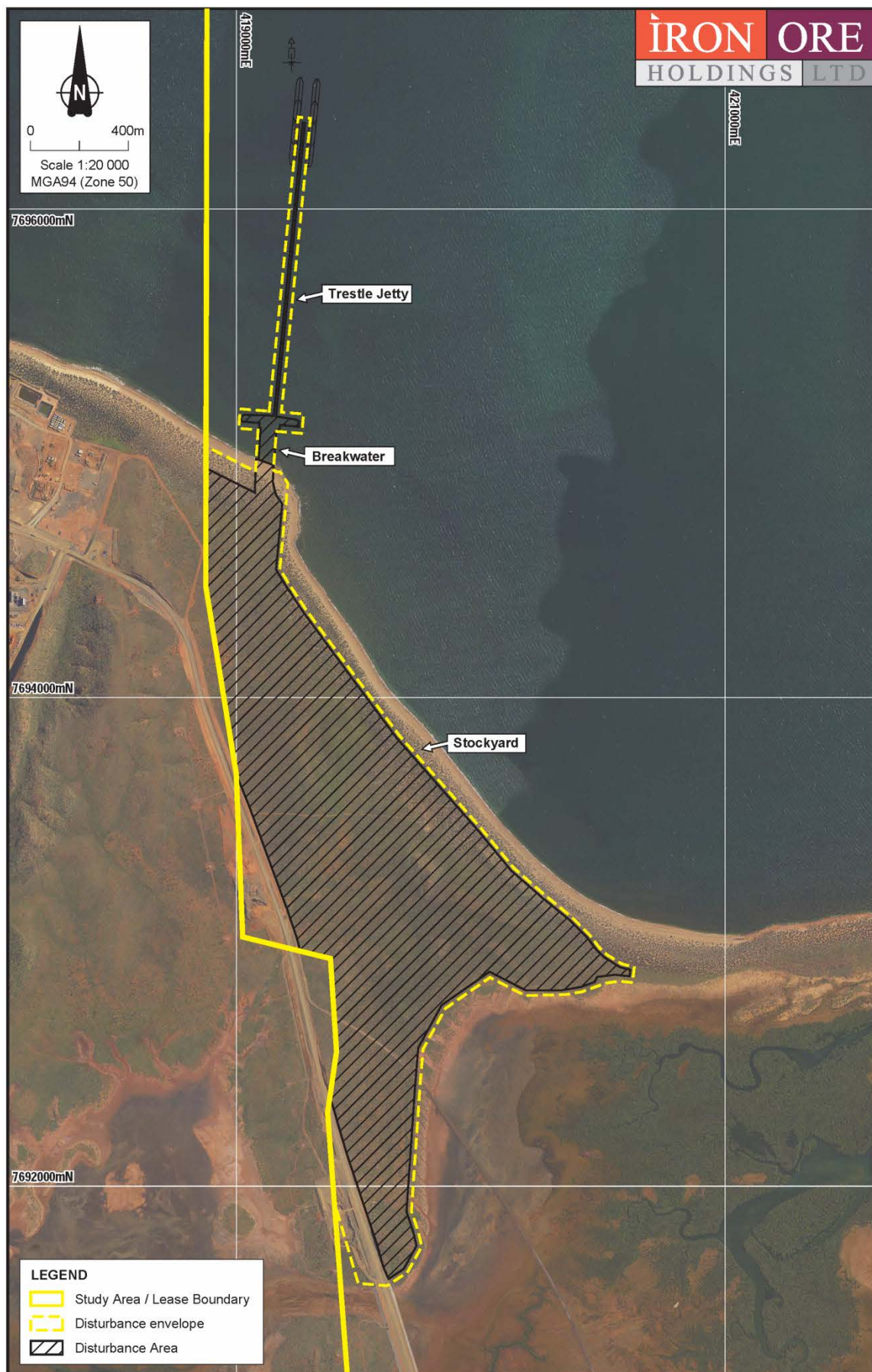
Figure 2 Trestle jetty and rock breakwater infrastructure
