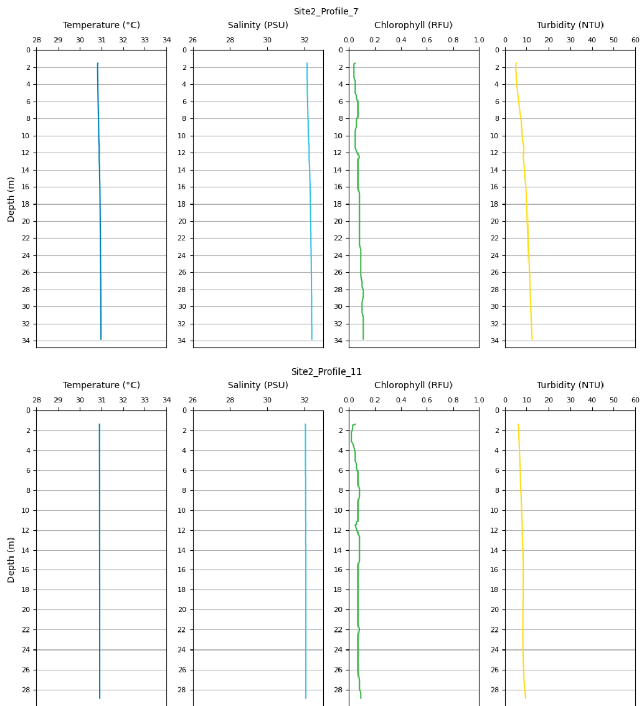
Figure 106. Measured temperature, salinity, chlorophyll and turbidity through the water column at Site 2 at high water (top) and during the ebb stage of the tide (bottom).
