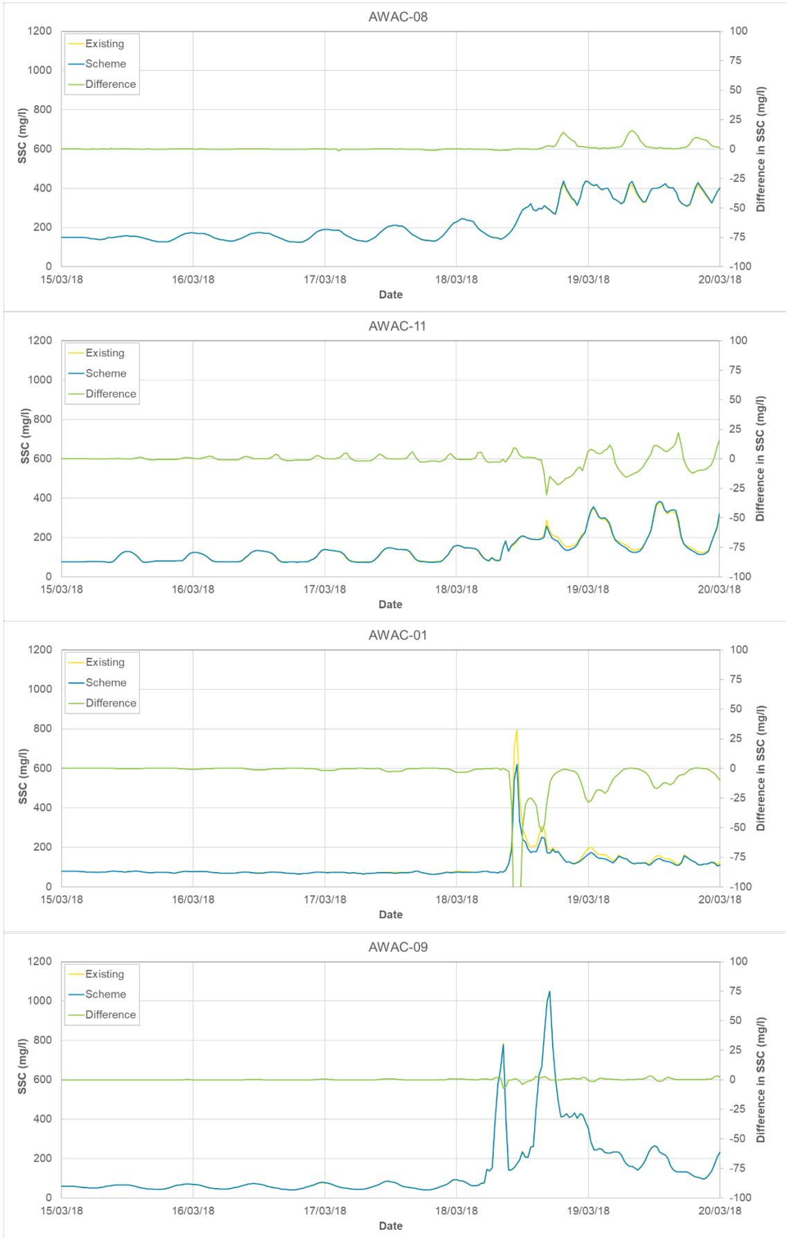
**Figure 205. Timeseries showing the modelled change in SSC during TC Marcus due to 15 years (70 million m<sup>3</sup>) of sand sourcing (Scheme).**
