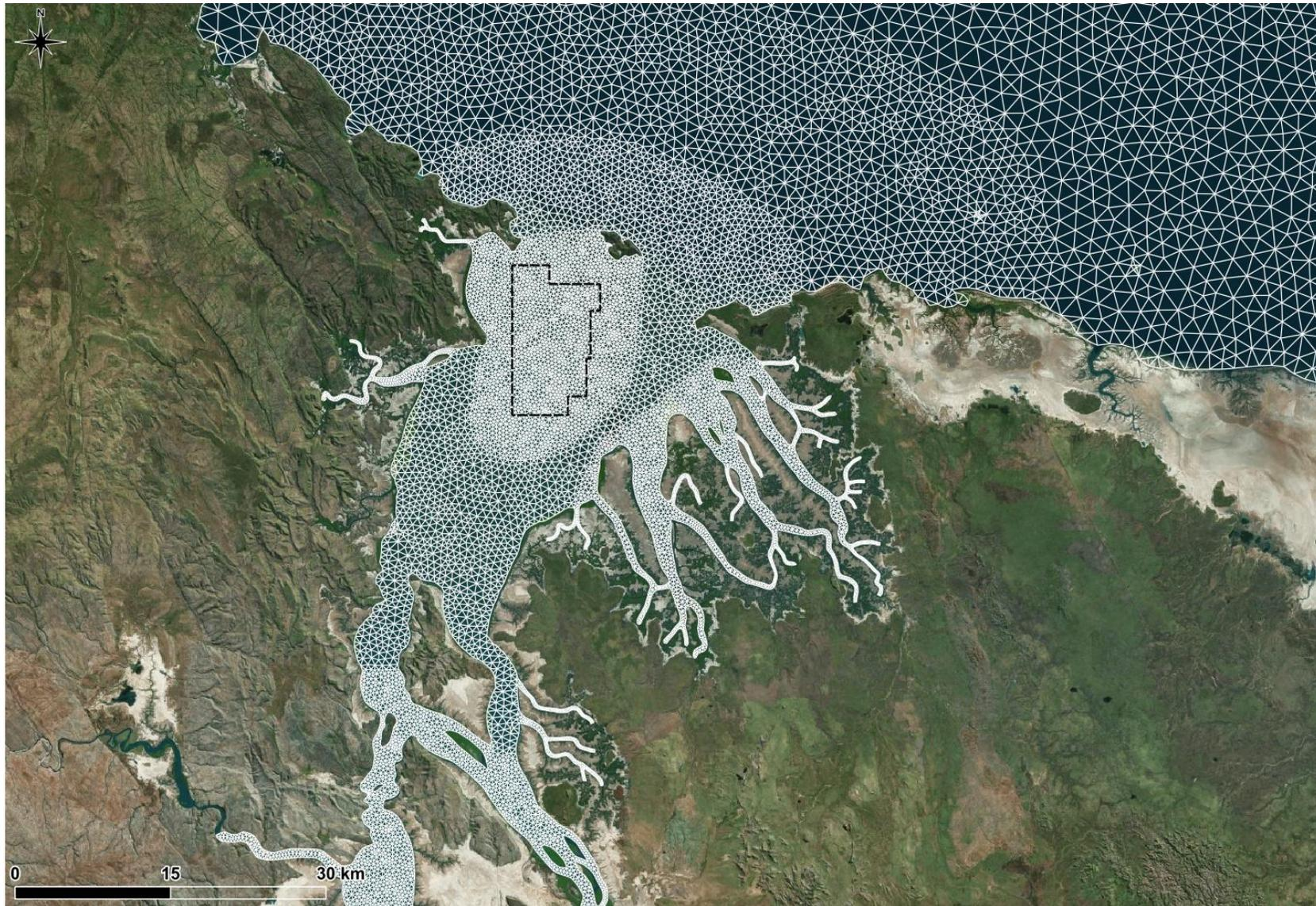
Figure 71. Close up of the numerical model mesh in CG along with Blocks 4 and 4A (grey polygons) and the proposed operational area (black dashed polygon).
