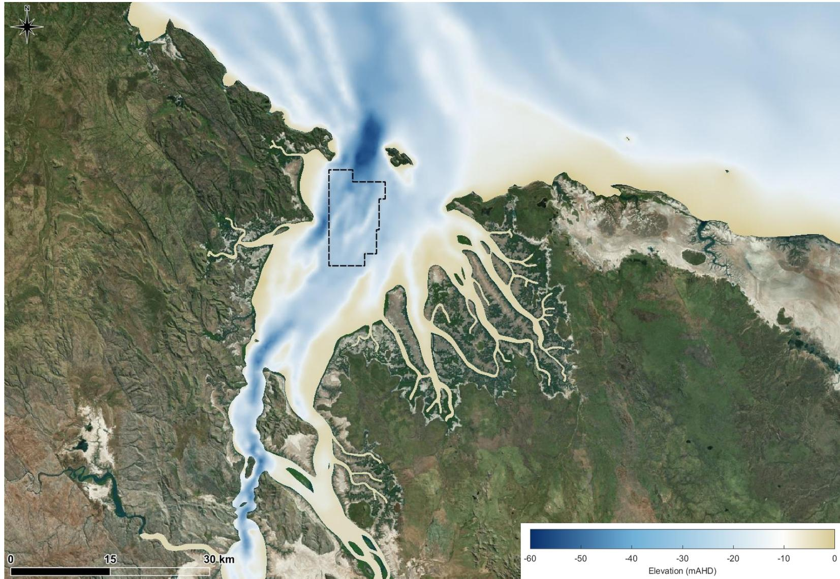
**Figure 73.** Model bathymetry for CG with Blocks 4 and 4A also shown (grey polygons) and the proposed operational area (black dashed polygon).
