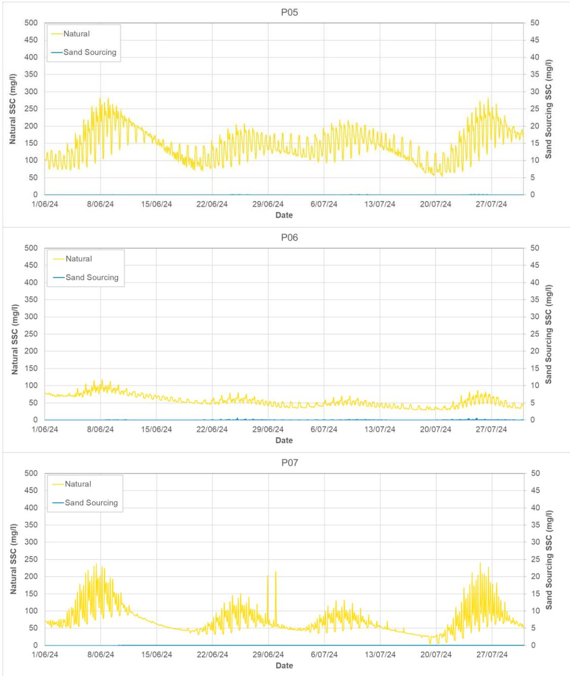
**Figure 244.** Timeseries showing the modelled natural SSC and sand sourcing SSC at P05 to P07 during the dry season for Scenario 1 with releases during spring tides. *Note: the sand sourcing SSC is plotted using a second y-axis with a lower SSC magnitude.*
