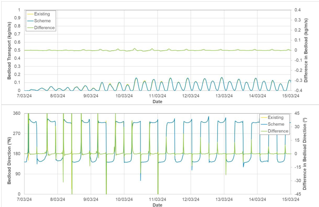
**Figure 218.** Timeseries showing the modelled difference in bedload transport rate (top) and direction (bottom) at AWAC-09 during a high river discharge event in the wet season in the pre-European scenario (Scheme) compared to the existing case.
