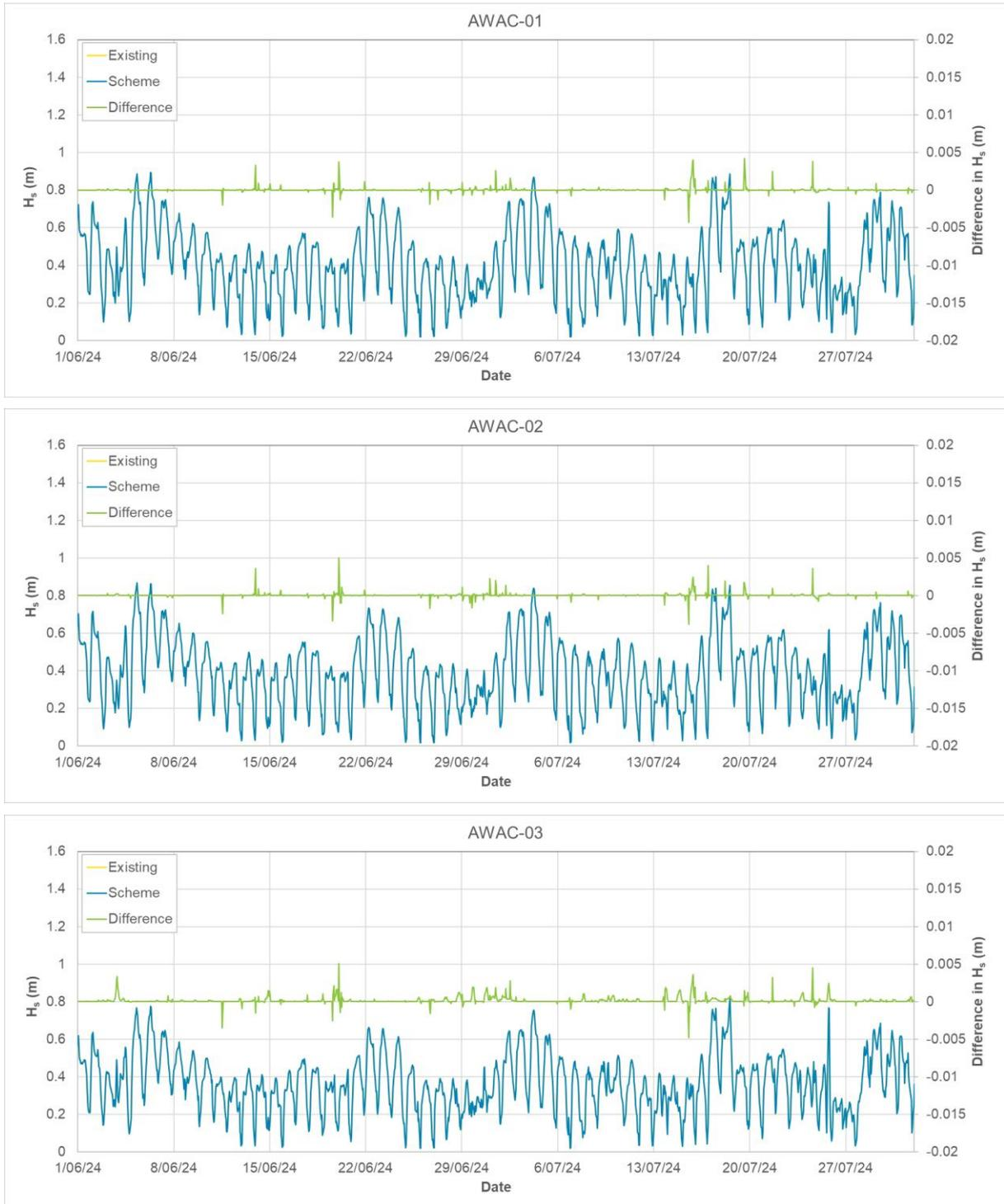
**Figure 159.** Timeseries showing the modelled change in  $H_s$  over the two-month (61 days) dry season simulation due to 15 years of sand sourcing (Scheme) at sites AWAC-01 to AWAC-03.
