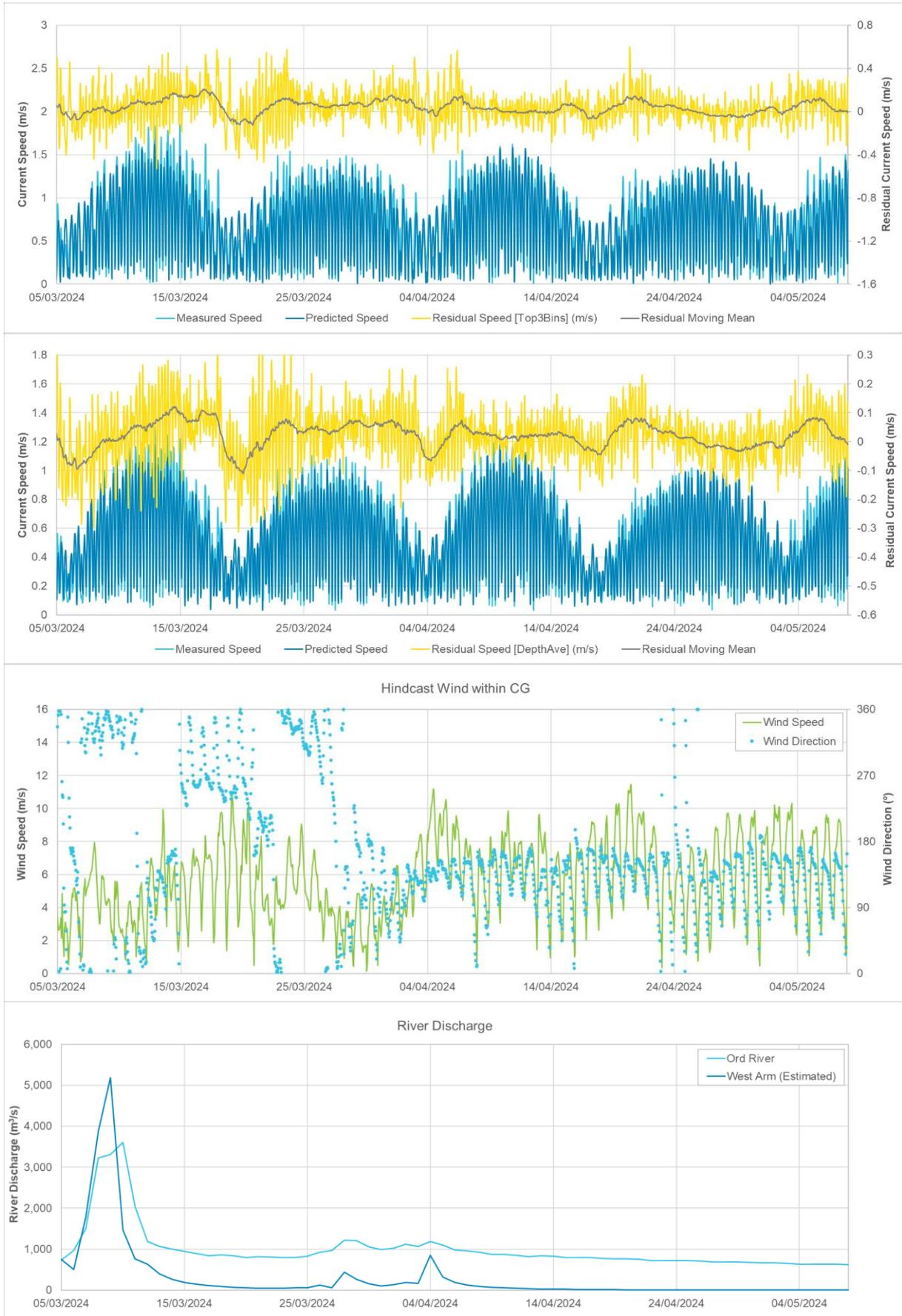
**Figure 23. Current residuals at AWAC-09 for surface (top) and depth-averaged (second) currents, hindcast modelled wind and measured river discharge during the wet season.**
