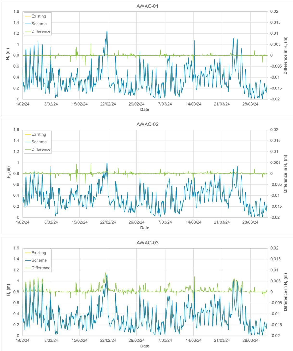
**Figure 157. Timeseries showing the modelled change in  $H_s$  over the two-month (60 days) wet season simulation due to 15 years of sand sourcing (Scheme) at sites AWAC-01 to AWAC-03.**
