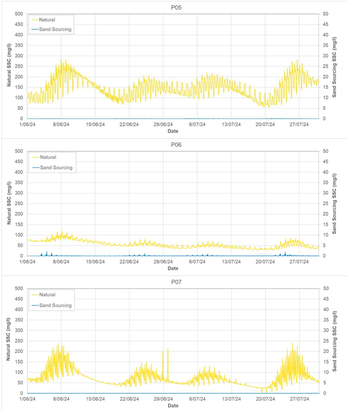
**Figure 241.** Timeseries showing the modelled natural SSC and sand sourcing SSC at P05 to P07 during the dry season for Scenario 1 with releases during neap tides. *Note: the sand sourcing SSC is plotted using a second y-axis with a lower SSC magnitude.*
