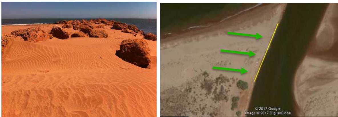
Figure 6.11: Aeolian transport assessment. (left) Sand overlaying the training wall (Seashore 2017), (right) exposed beach width and entry point into Beadon Creek
