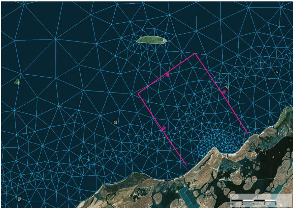
Figure 3.7: Local Model Domain (shown in magenta) nested inside Regional Model Domain Flexible Mesh Grid (shown in Blue)
