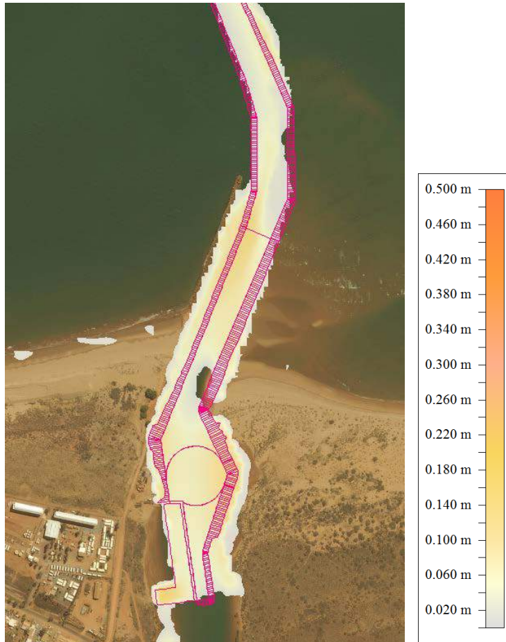
Figure A.10: Fines Accumulation – total annual sedimentation for Channel Entrance and OMSB area
