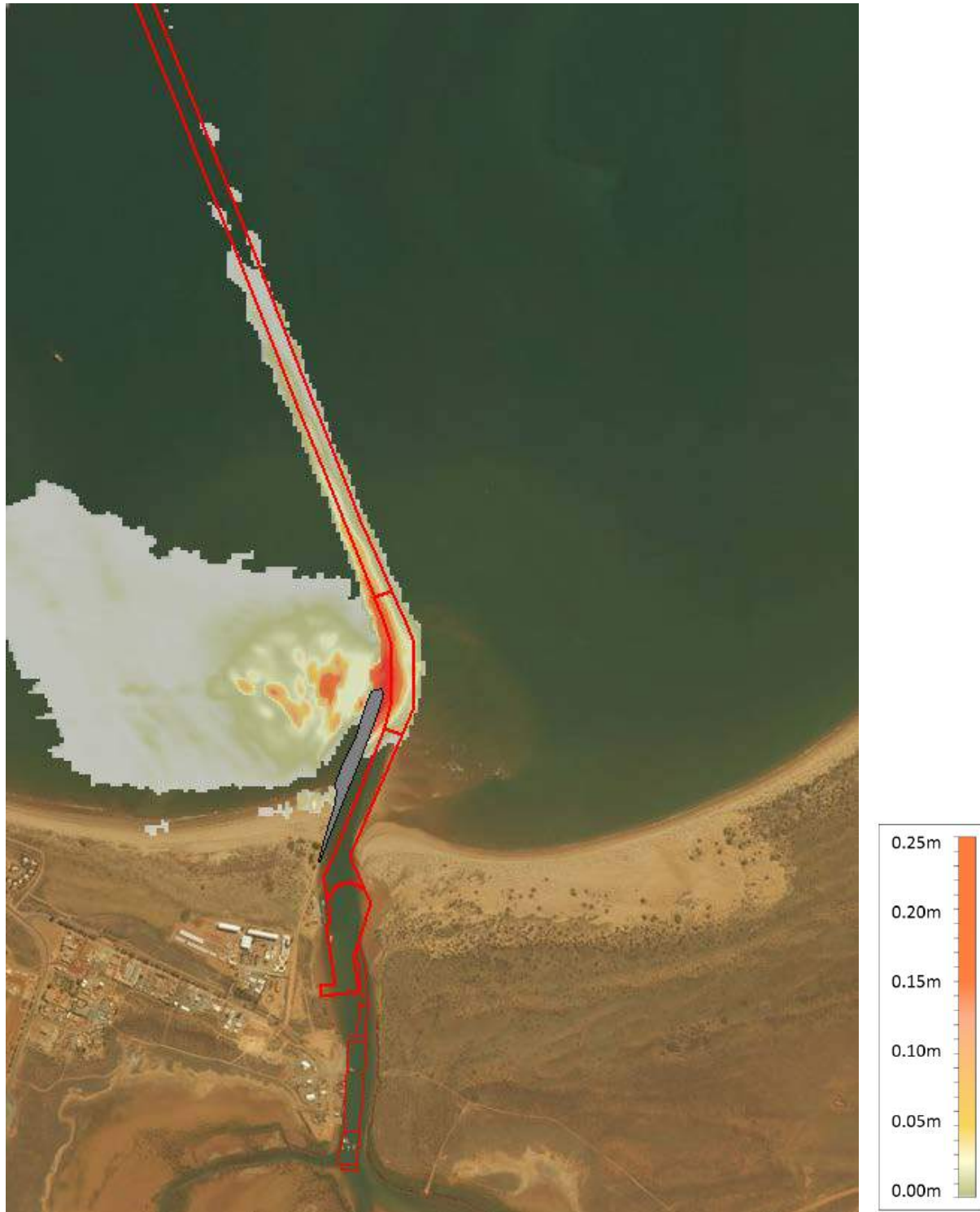
Figure A.8: Distribution of Littoral Drift Volume that Bypasses the Training Wall Structure under developed conditions
