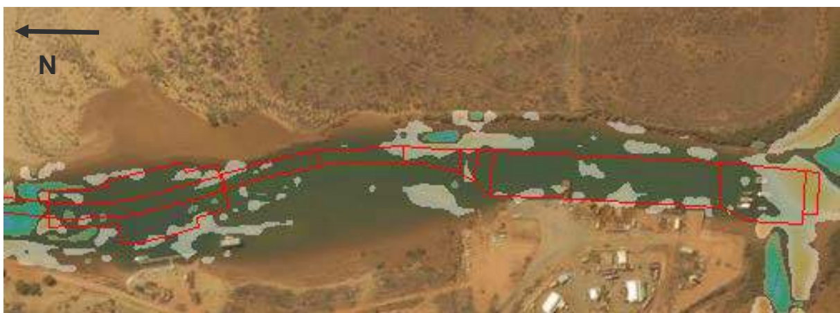
Figure A.13: Modelled annual erosion and sedimentation for the existing case. Outer channel (upper) and inside Beadon Creek (lower) areas with channel sections overlaid.
