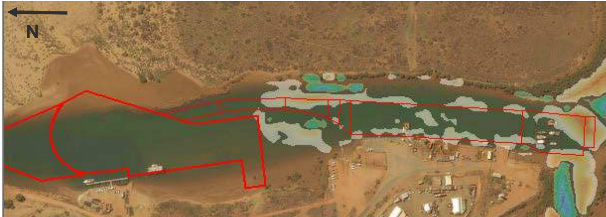
Figure 6.17: Modelled annual erosion and sedimentation for the developed case inside Beadon Creek with channel sections overlaid
