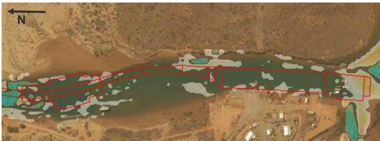
Figure 6.13: Modelled annual erosion and sedimentation for the existing case. Outer channel (upper) and inside Beadon Creek (lower) areas with channel sections overlaid.
